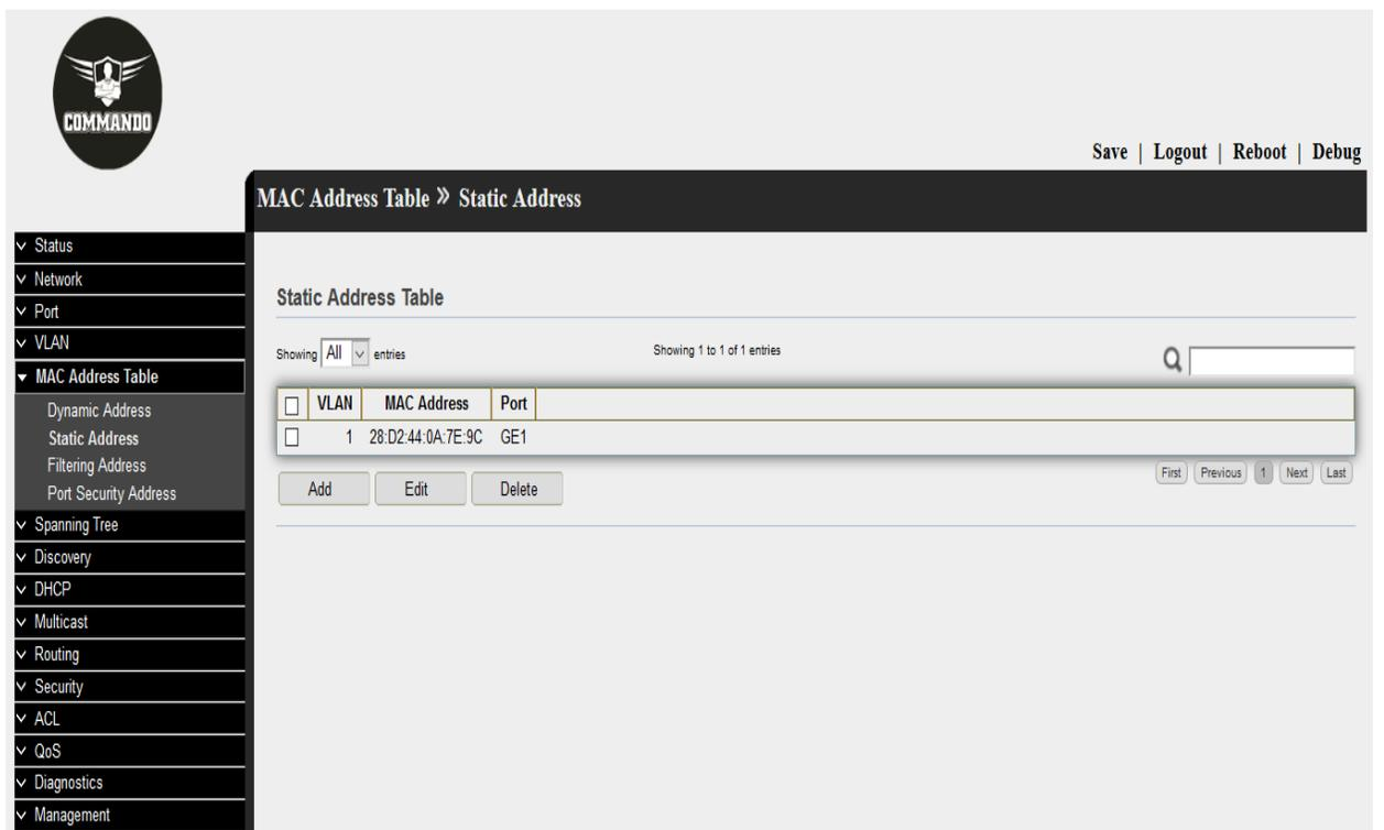
Fig 6.2.3 Static MAC address table After adding MAC address page
