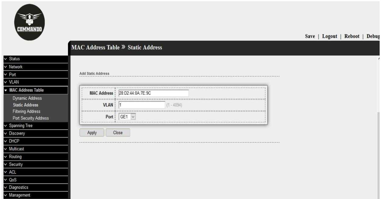
Fig 6.2.2 Add Static MAC address to specified VLAN and port page
