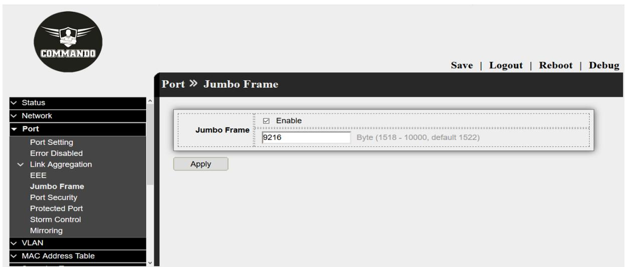
Fig 4.5.2 Jumbo Frame Enable for 9216 bytes page
