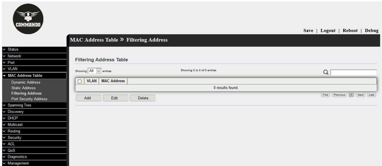
Fig 6.3.1 Filtering address table default page
