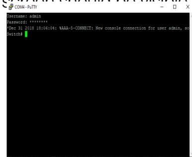
Fig 3. COMMANDO Series E2000 Switch CLI access via console port
