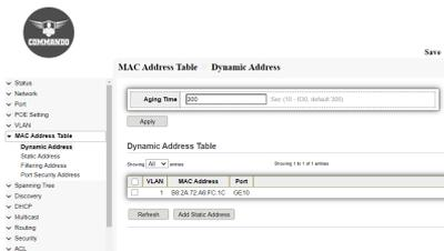
Fig 6.1.2 Add Static address from Dynamic MAC address table page
