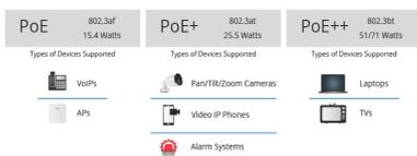
Fig 17.1 E2000 Series PoE/PoE+ Switches Concept
