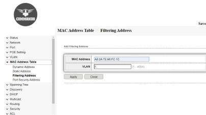
Fig 6.3.1 Filtering address table default page
