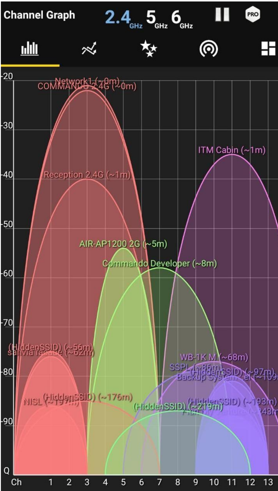
Fig 3.1.25 WiFi analysis 2.4G band of AIR-AP01200
