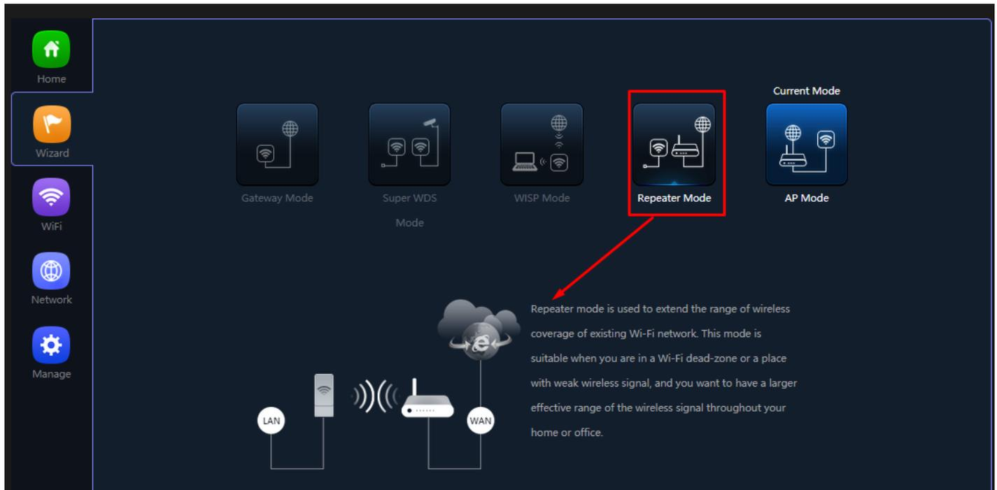
**Fig 2.4.1 Repeater mode of AirONE APO300**
