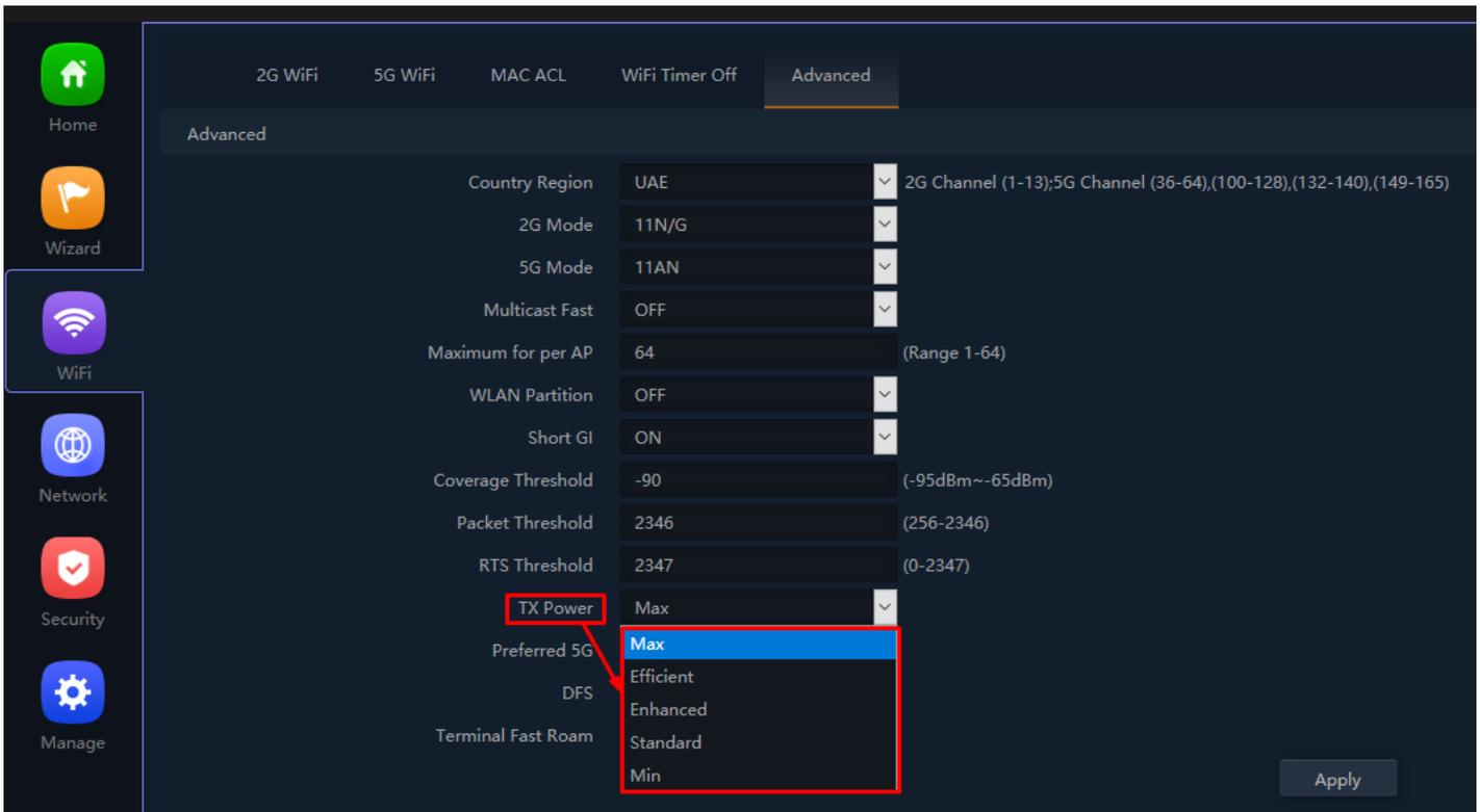
Fig 3.5.10 Setting Tx Power for AirONE APO750
