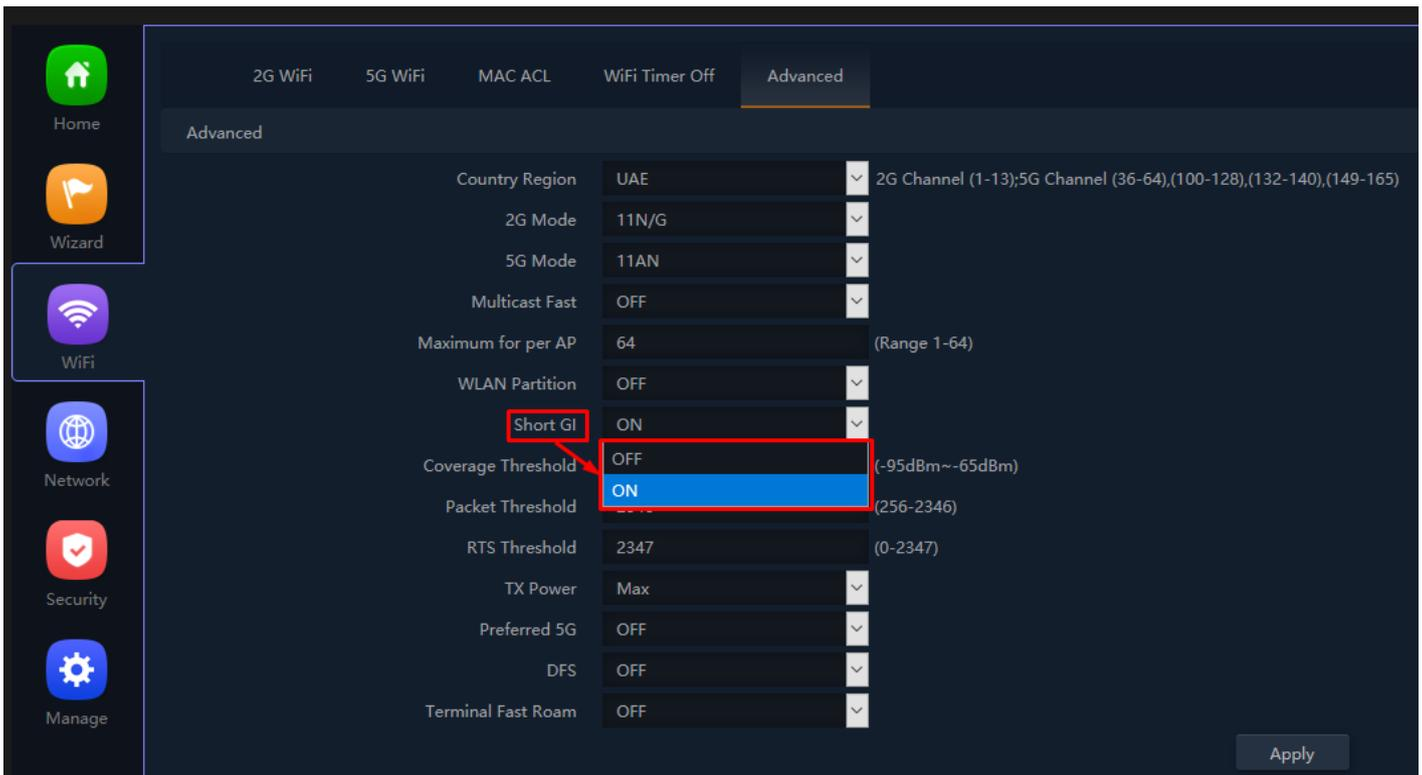
**Fig 3.5.8 Selecting Short GI for AirONE APO750**
