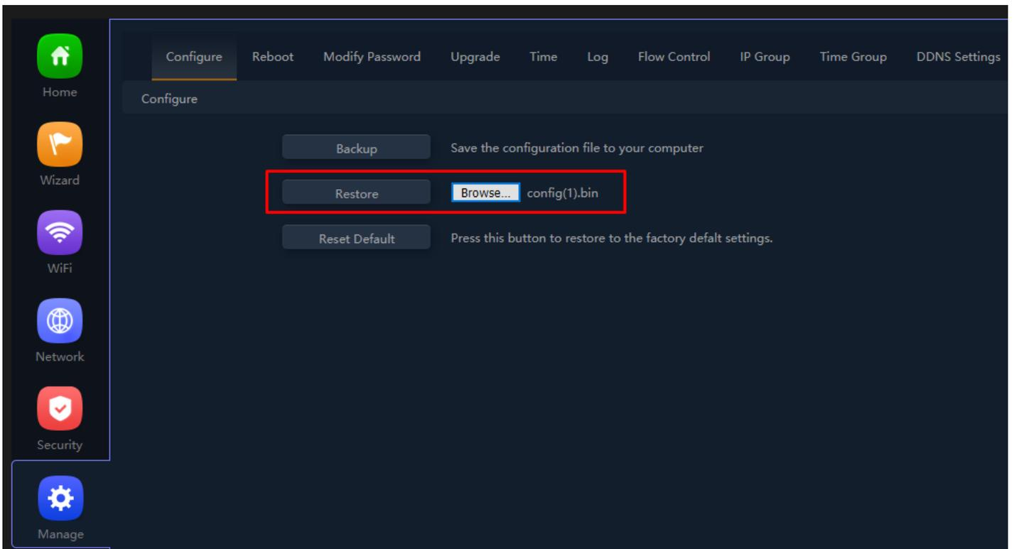
**Fig 6.1.3 Restore to known Configure for AirONE APO750**
