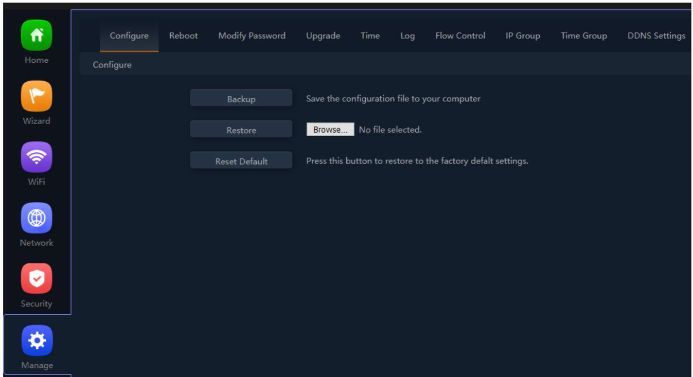
**Fig 6.1.1 Default Configure setting for AirONE APO750**
