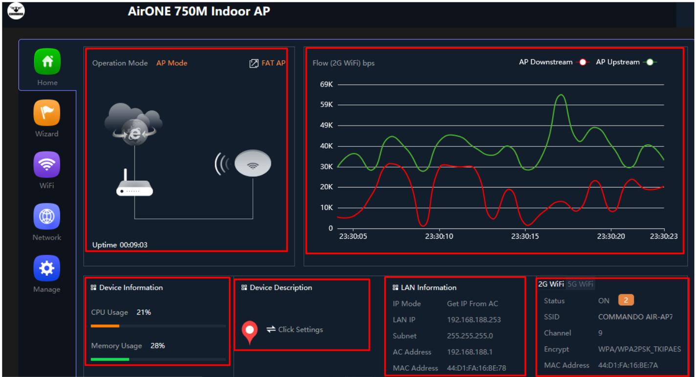
**Fig 1.1 Home page Components of AirONE APO750** (This image is for reference purpose only)
