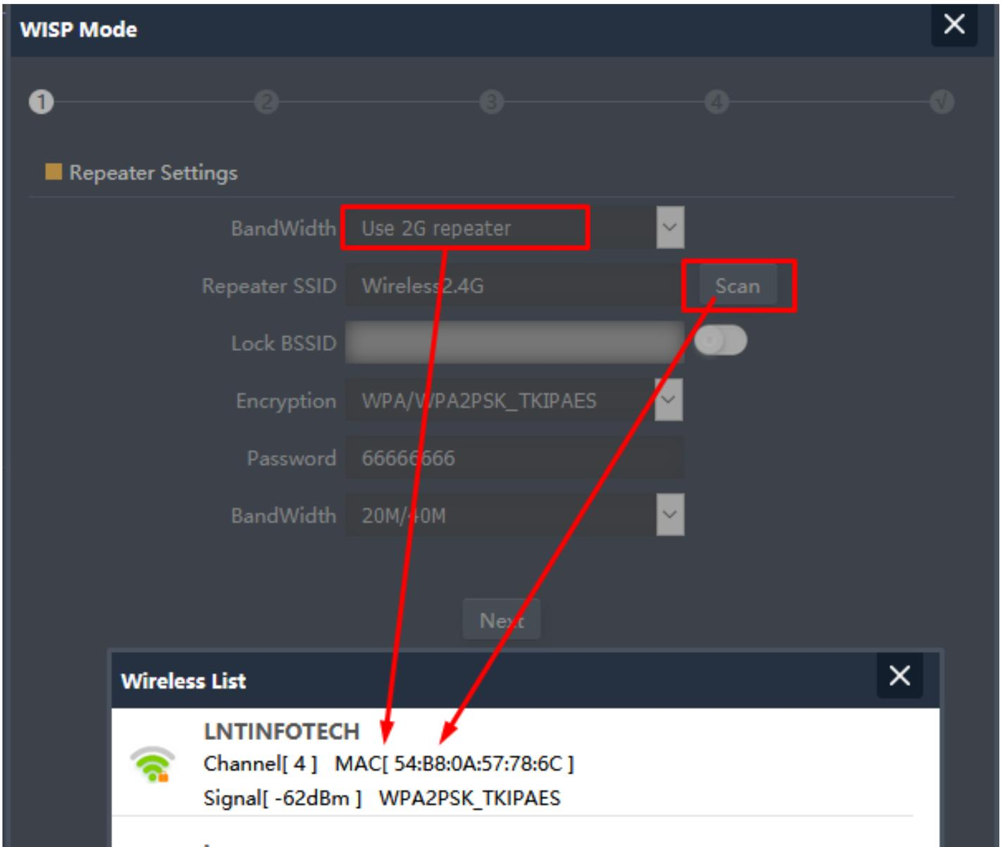
Fig 2.3.2 2G Repeater Setting WISP mode of AirONE APO750
