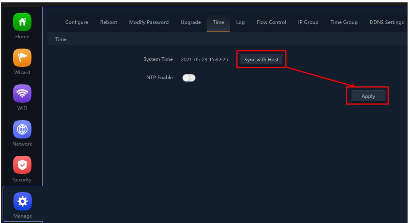
**Fig 6.5.2 Disable NTP and Sync with host for AirONE APO750**
