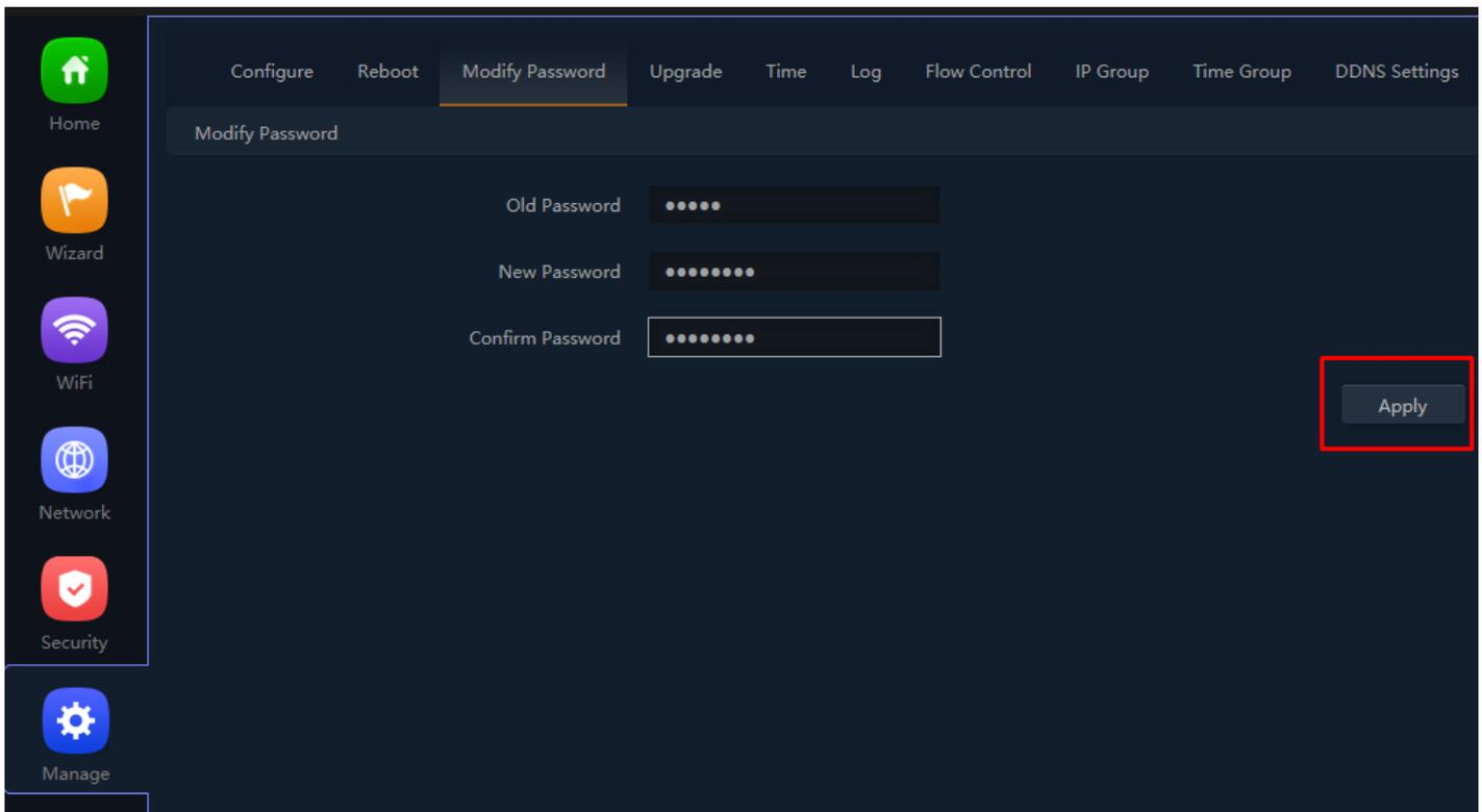
**Fig 6.3.2 Setting New password for AirONE APO750**
