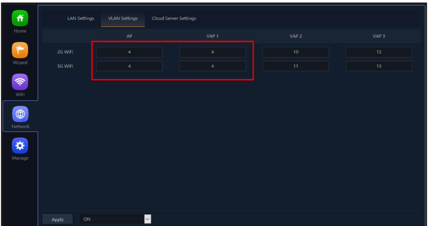
**Fig 4.2.2 VLAN setting for AirONE APO750**
