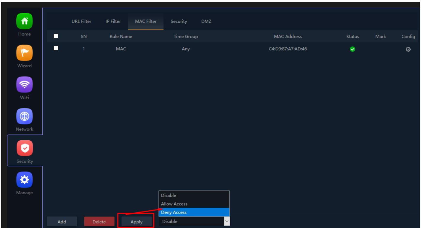
**Fig 5.3.3 MAC filter setting for AirONE APO750**
