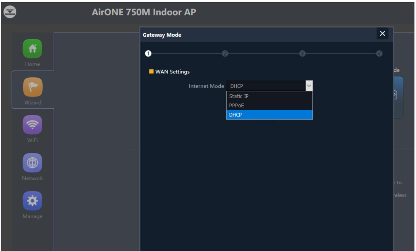
Fig 2.1.2 Gateway mode WAN Setting of AirONE APO750
