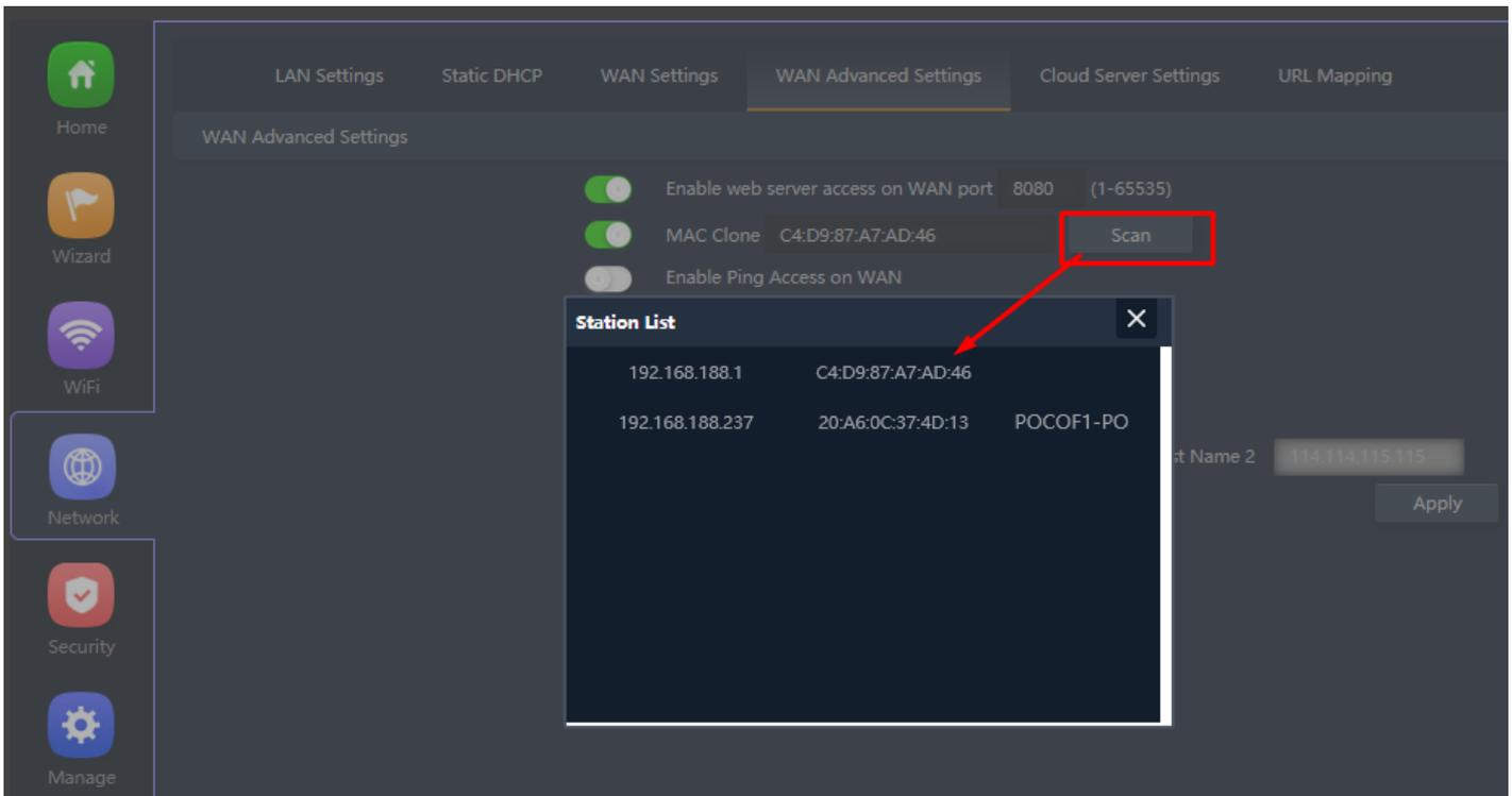
**Fig 4.5.3 Configuration of MAC clone for AirONE APO750**
