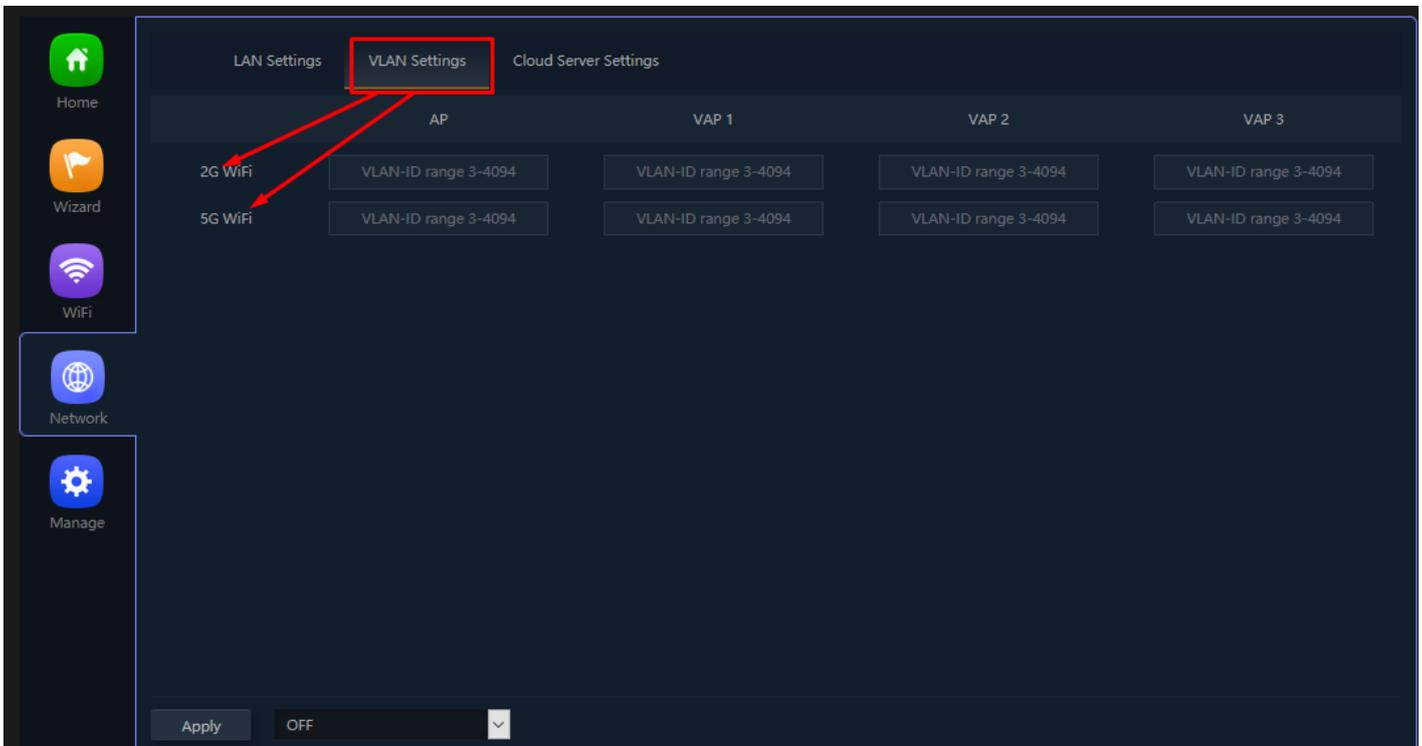
**Fig 4.2.1 Default VLAN setting for AirONE APO750**
