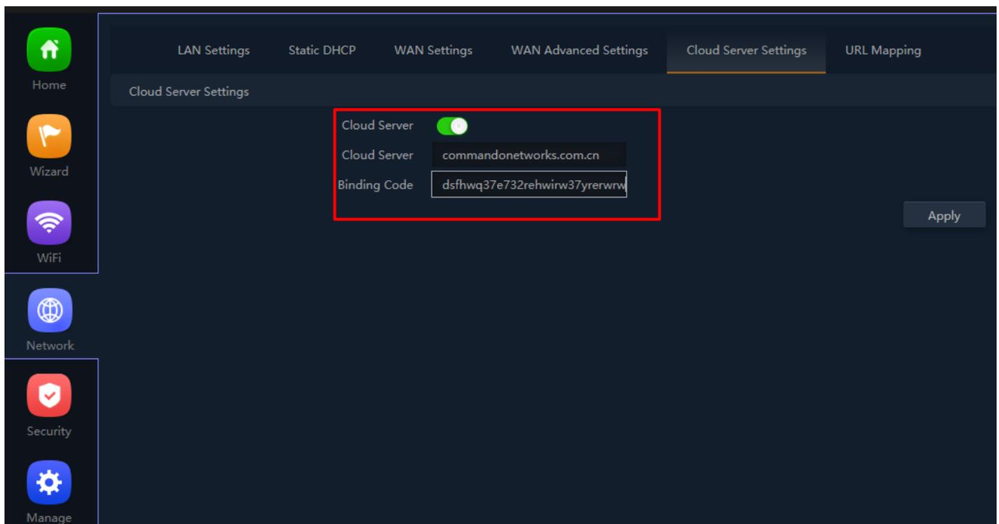
**Fig 4.6.2 Enabling Cloud server setting for AirONE APO75**
