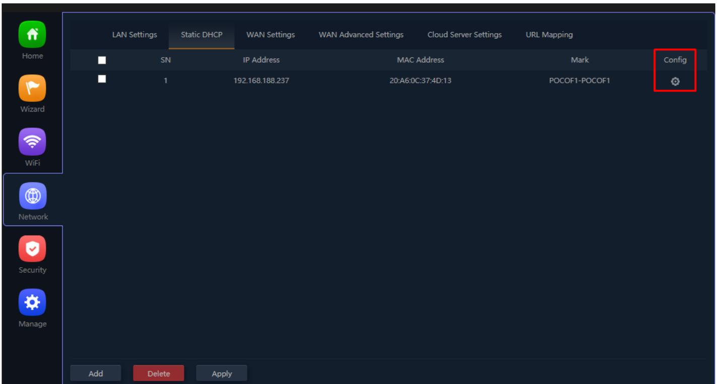
Fig 4.3.4 Static DHCP for AirONE APO750
