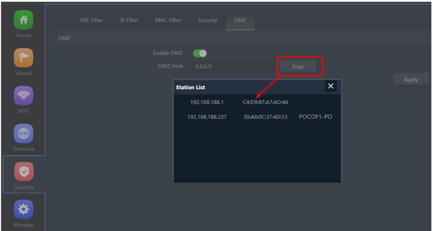
**Fig 5.5.2 DMZ setting for AirONE APO750**
