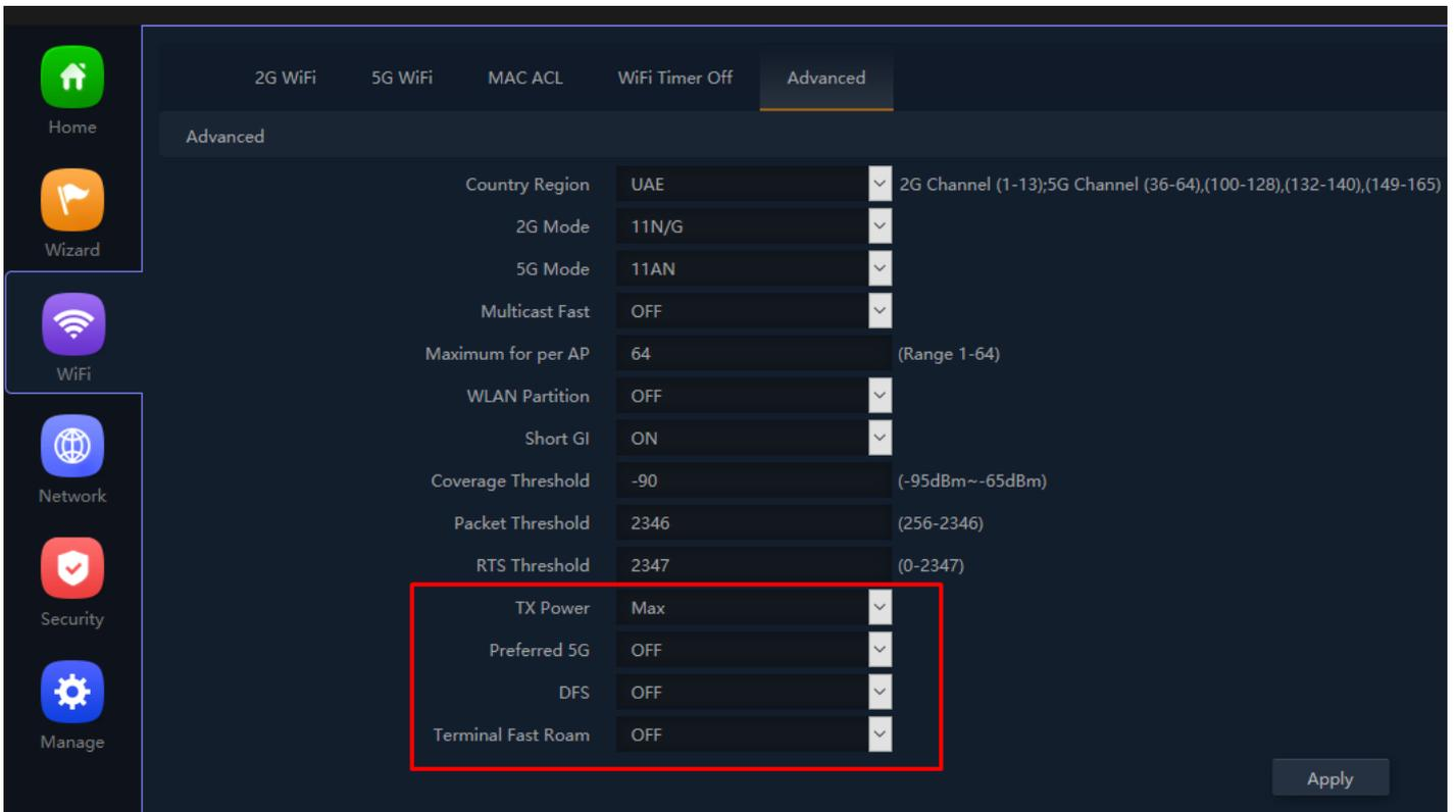
**Fig 3.5.11 Setting Preferred 5G, DFS, Terminal Fast Roam for AirONE APO750**
