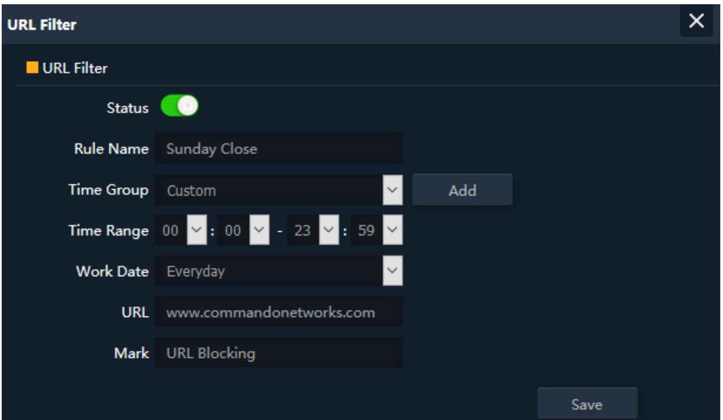
Fig 5.1.2 Setting URL filter for AirONE APO750
