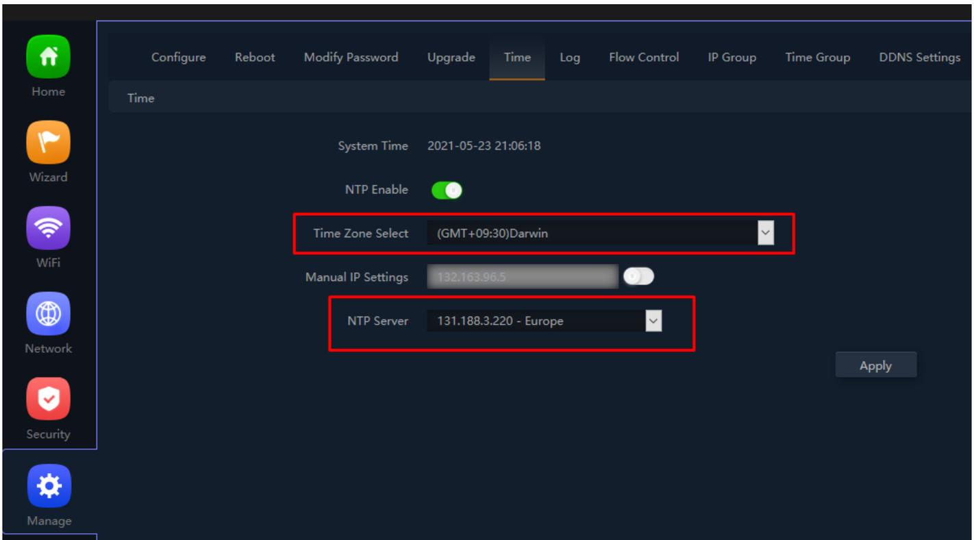
Fig 6.5.6 NTP server for AirONE APO750
