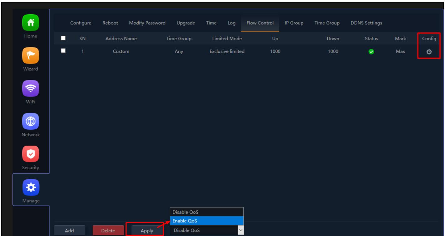
Fig 6.7.3 Flow control page for AirONE APO750
