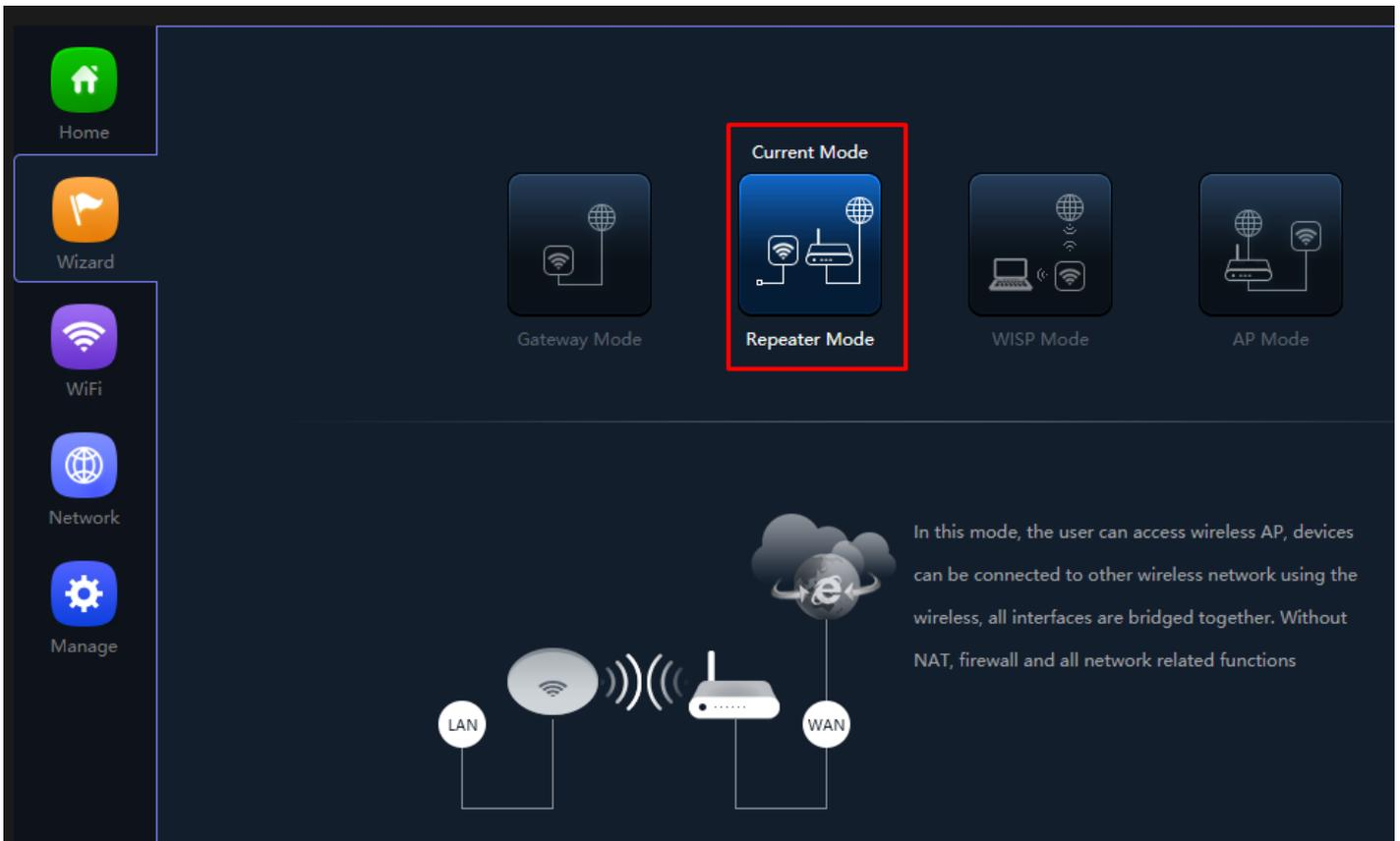
**Fig 2.3.1 Repeater mode of AirONE APO750**
