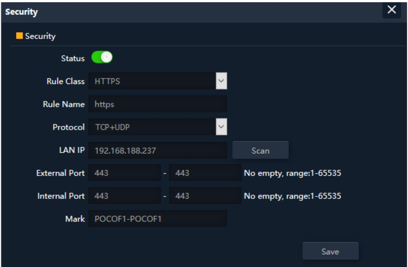
Fig 5.4.2 Security Rules setting for AirONE APO750
