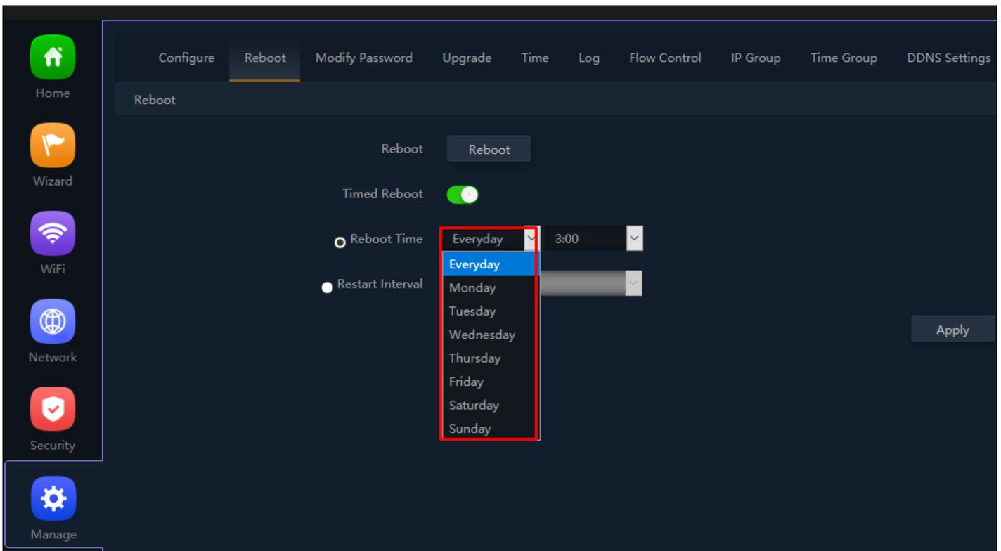
**Fig 6.2.3 Enable timed reboot for AirONE APO750**
