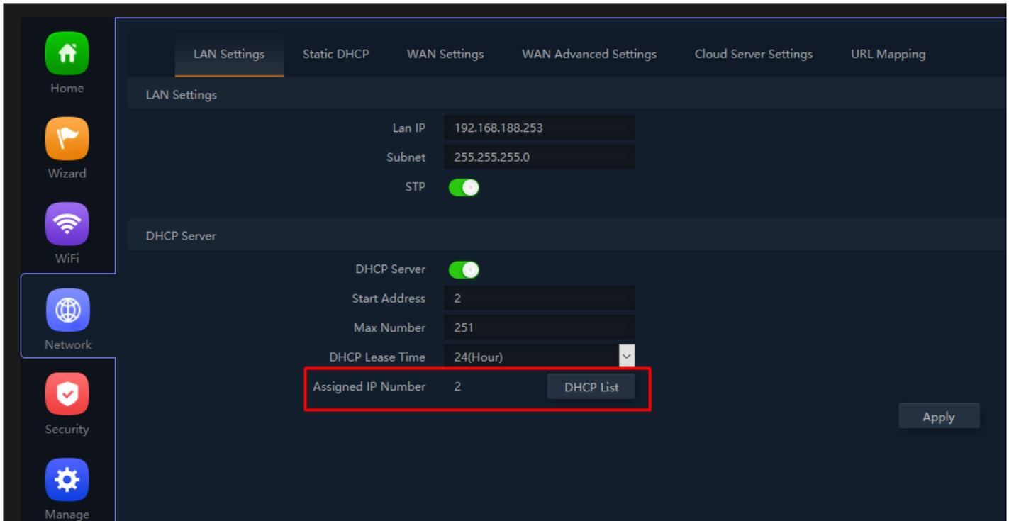
**Fig 4.1.4 DHCP Assigned list for AirONE APO750**
