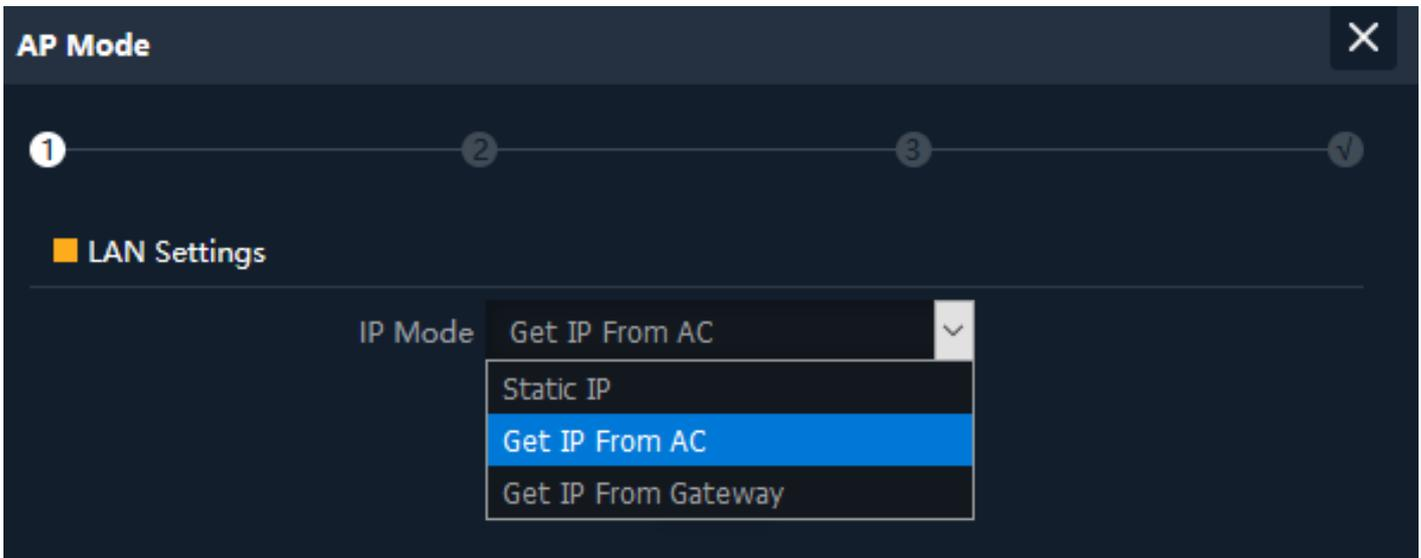
**Fig 2.4.2 Setting IP mode of AirONE APO750**
