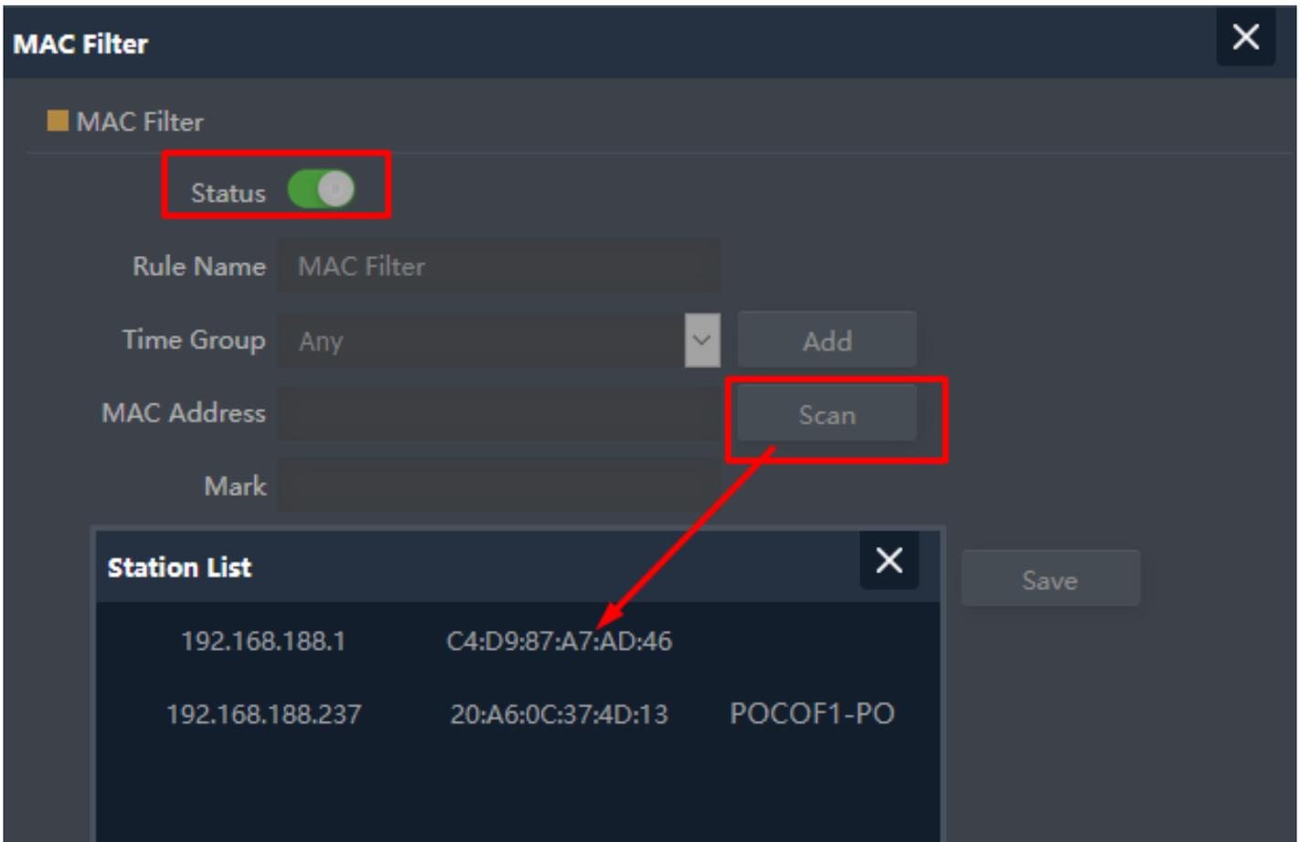
**Fig 5.3.2 Setting MAC filter for AirONE APO750**
