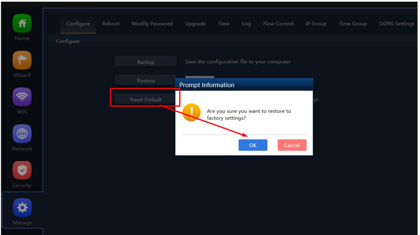
**Fig 6.1.4 Reset to factory default for AirONE APO75**
