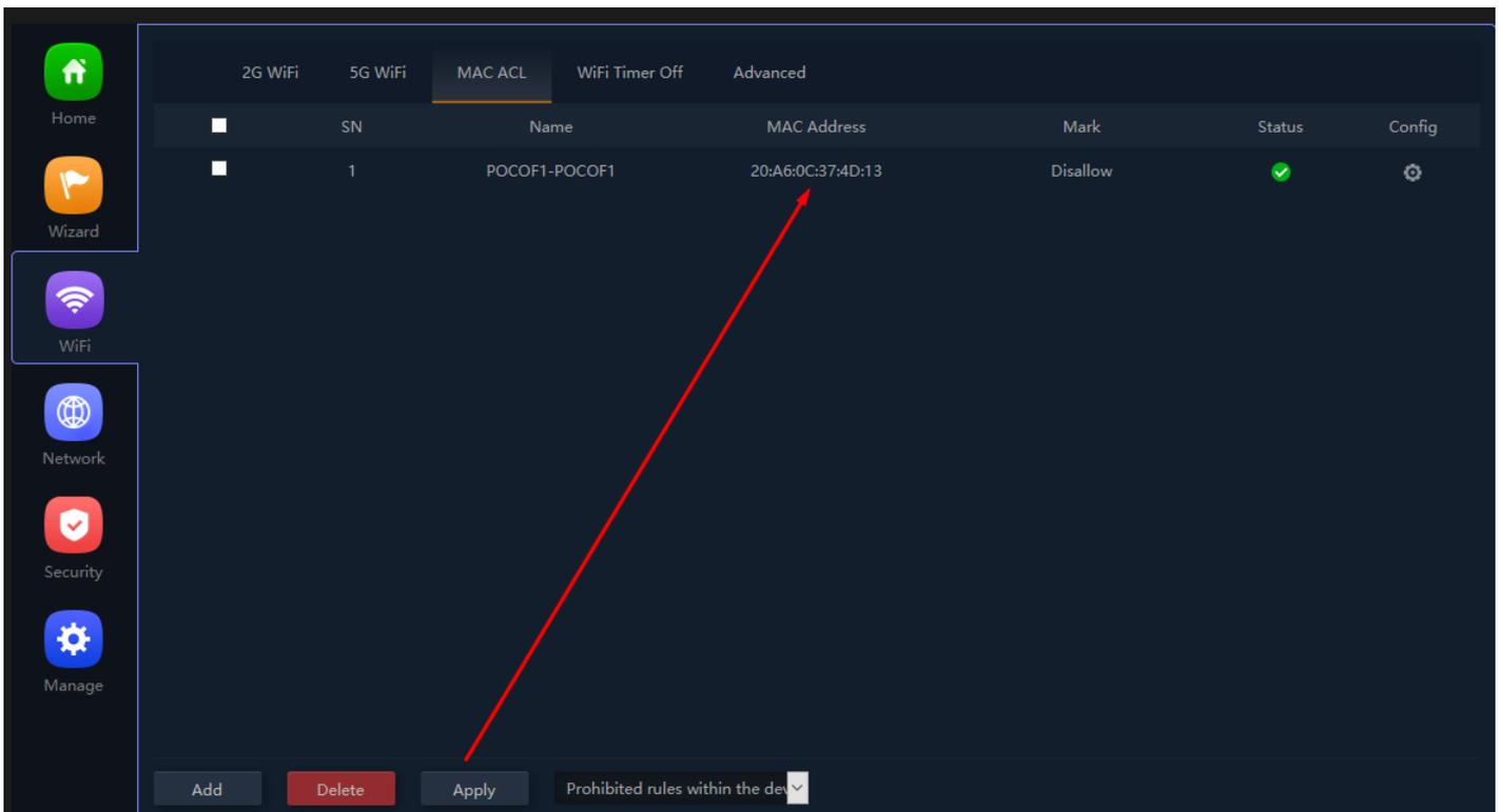
Fig 3.3.4 Apply MAC ACL for AirONE APO750
