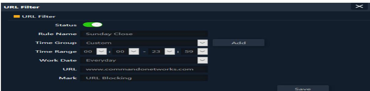
Fig 6.1.2 Setting URL filter for AirONE AIR-CPE1K+
