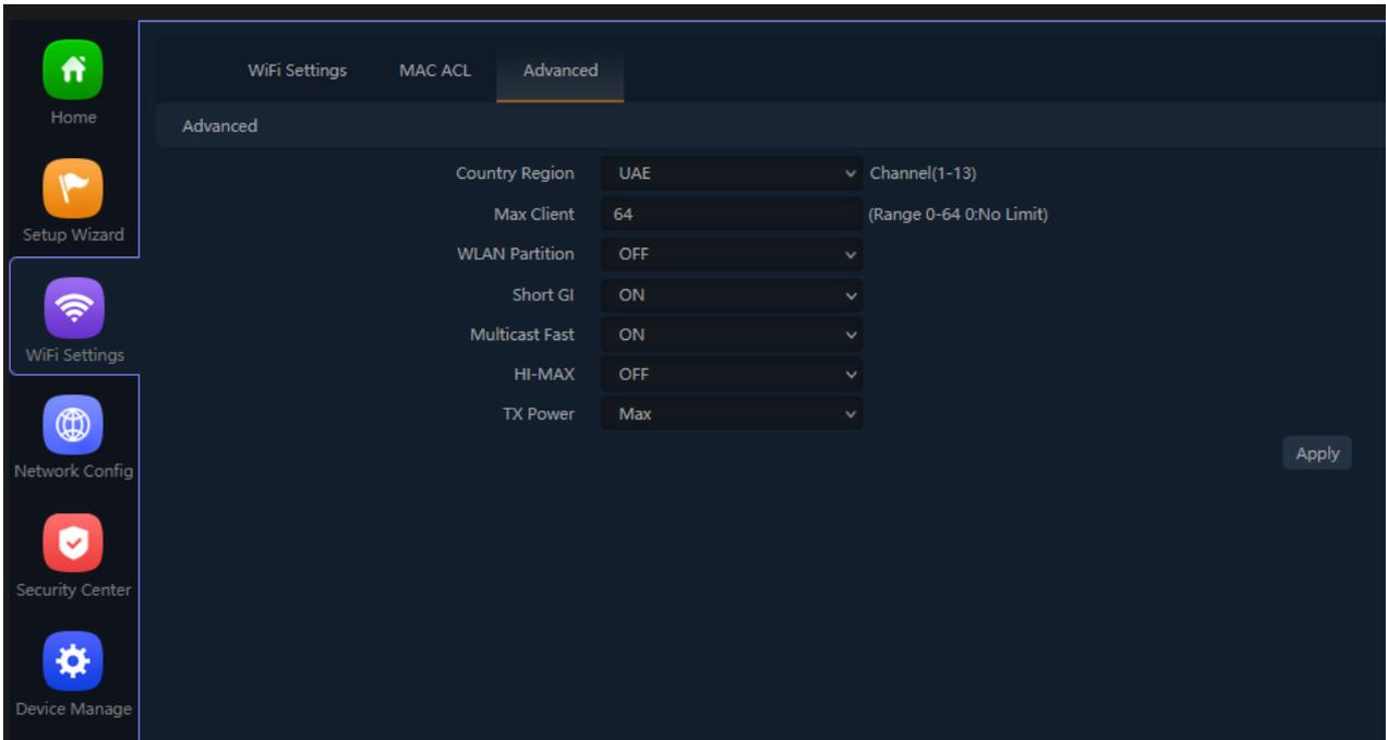
Fig 4.4.1 Default Advanced setting for AirONE AIR-CPE1K+
