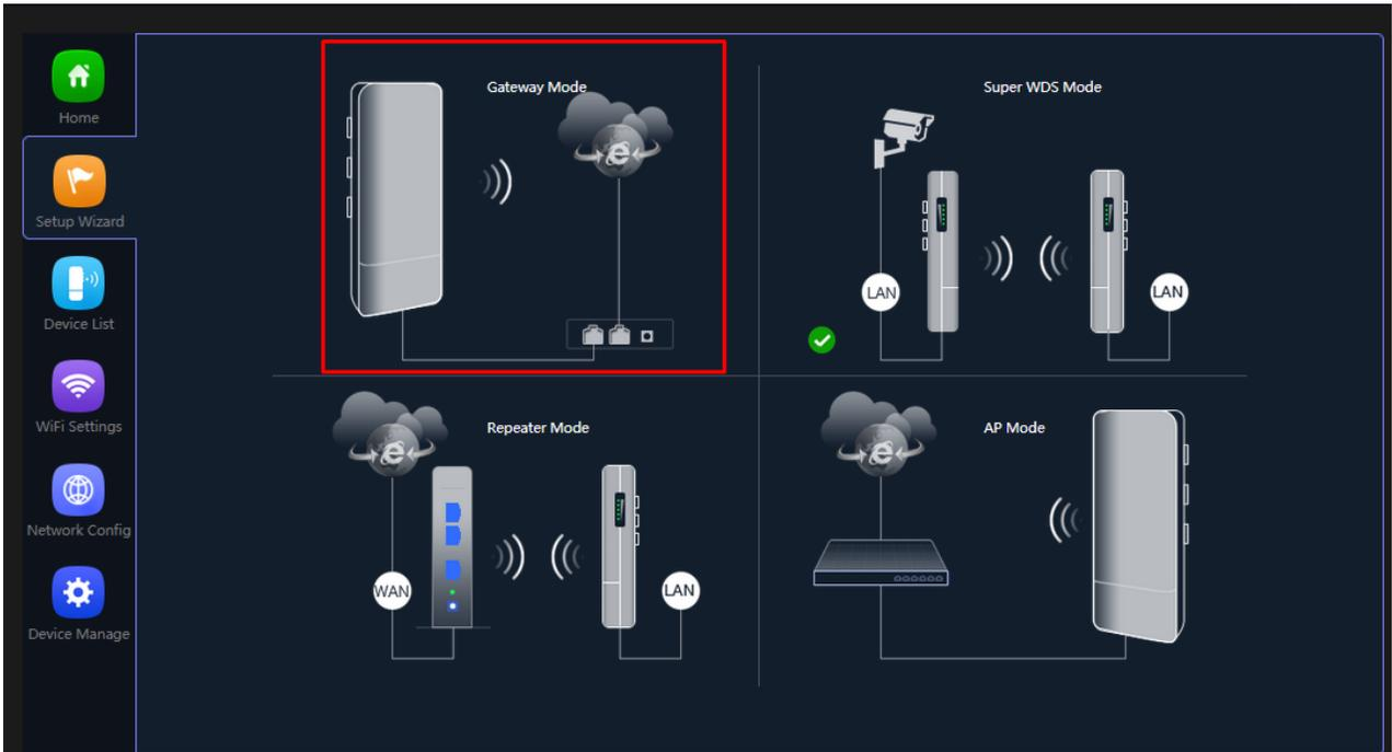
Fig 2.1.1 Gateway mode of AirONE AIR-CPE1K+
