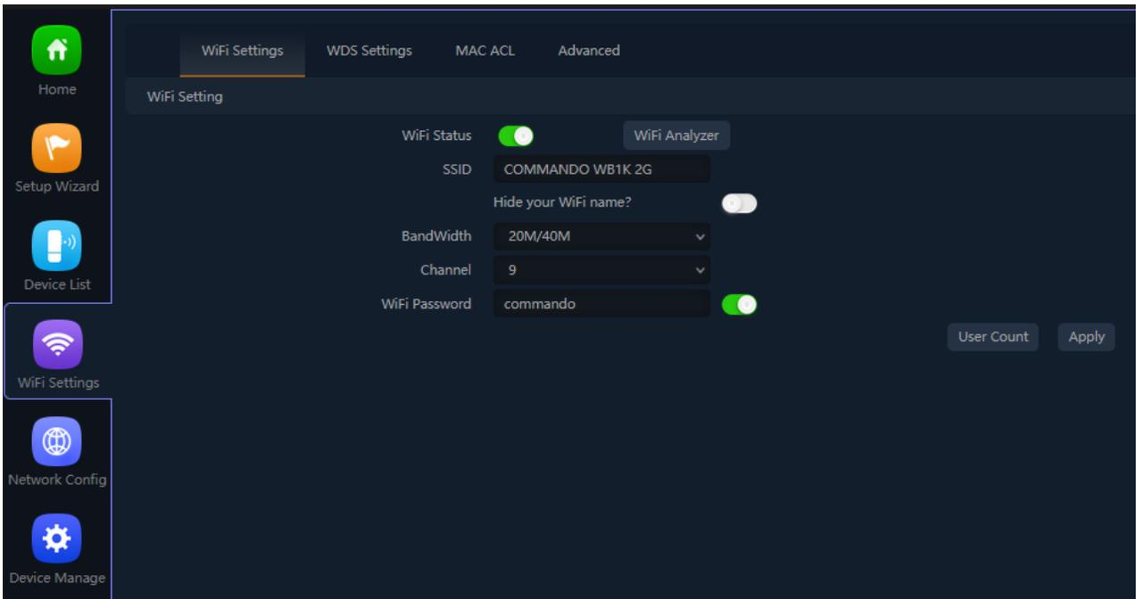
Fig 4.1.1 2G Basic Wi-Fi of AirONE AIR-CPE1K+
