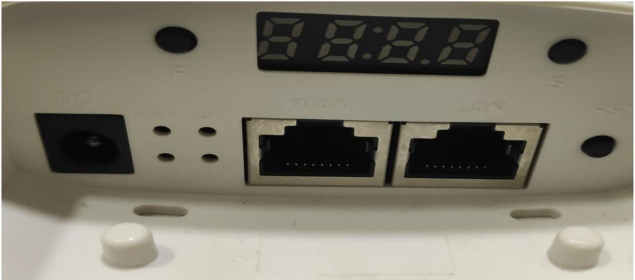
Fig 1. Physical port on AirONE AIR-CPE1K+
