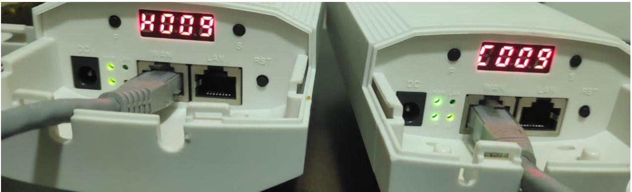
Fig 1. Physical port on AirONE AIR-CPE1K+
