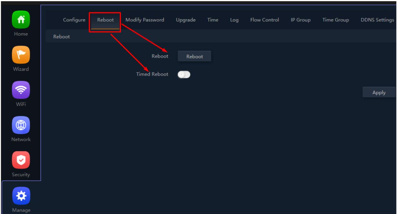
Fig 7.2.1 Default reboot setting for AirONE AIR-CPE1K+
