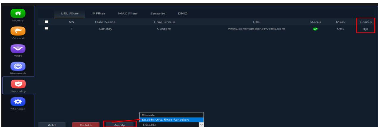
Fig 6.1.3 URL filter setting for AirONE AIR-CPE1K+
