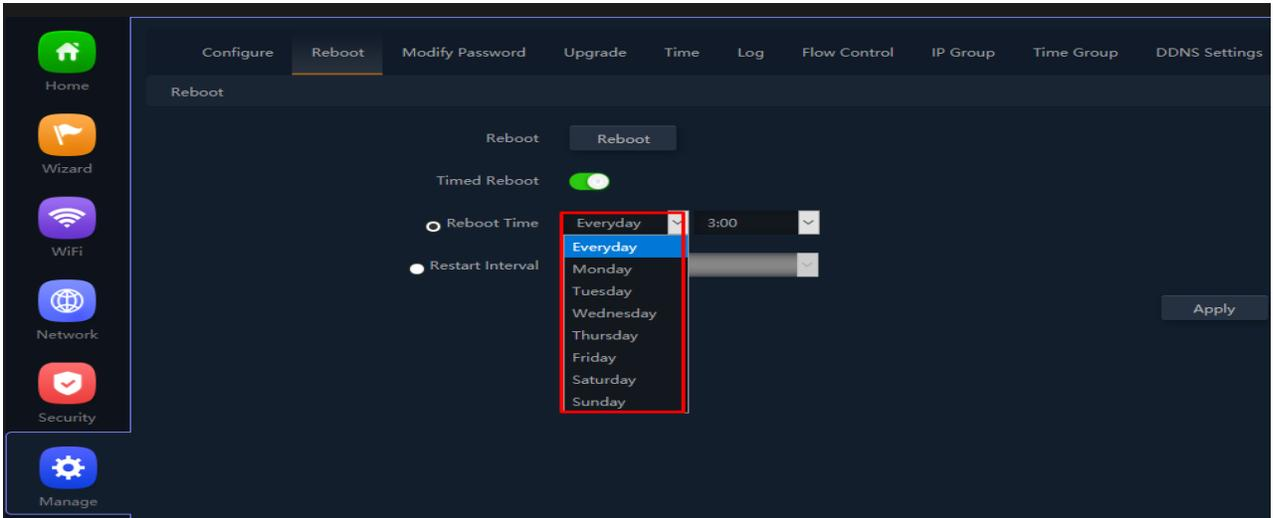
Fig 7.2.3 Enable timed reboot for AirONE AIR-CPE1K+
