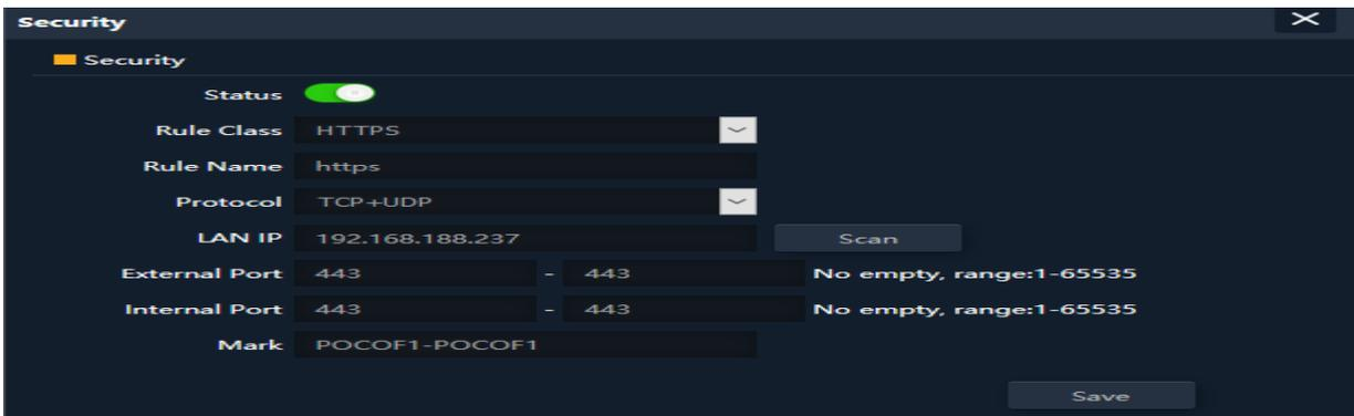
Fig 6.4.2 Security Rules setting for AirONE AIR-CPE1K+
