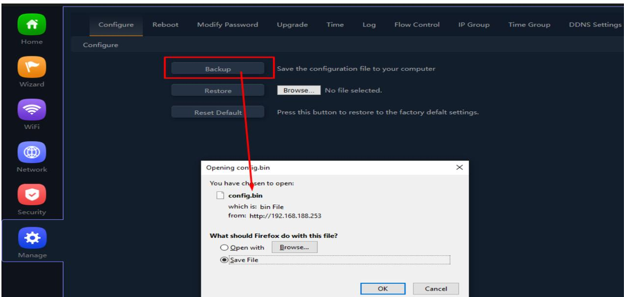
Fig 7.1.2 Taking backup of AirONE AIR-CPE1K+
