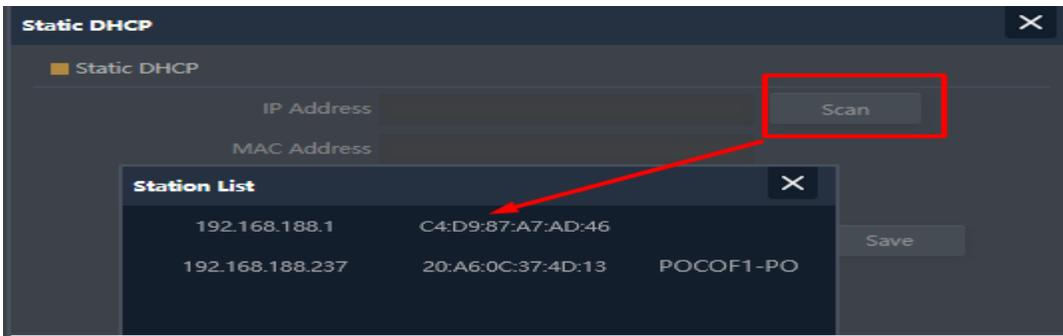
Fig 5.3.3 Station list for AirONE AIR-CPE1K+
