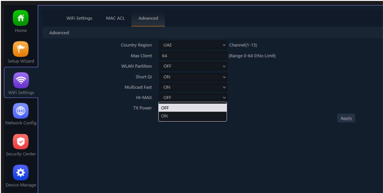
Fig 4.4.7 Selecting HI-MAX for AirONE AIR-CPE1K+
