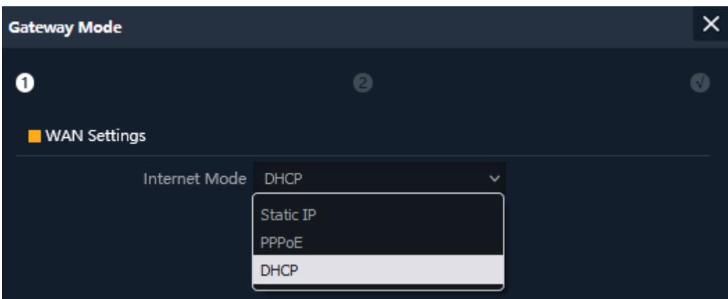
Fig 2.1.2 Gateway mode WAN Setting of AirONE AIR-CPE1K+
