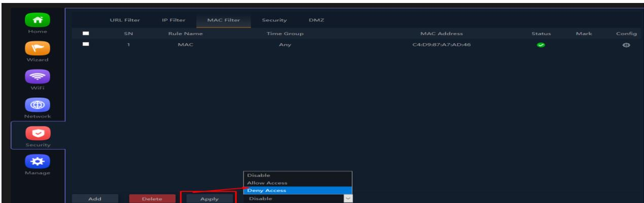
Fig 6.3.3 MAC filter setting for AirONE AIR-CPE1K+
