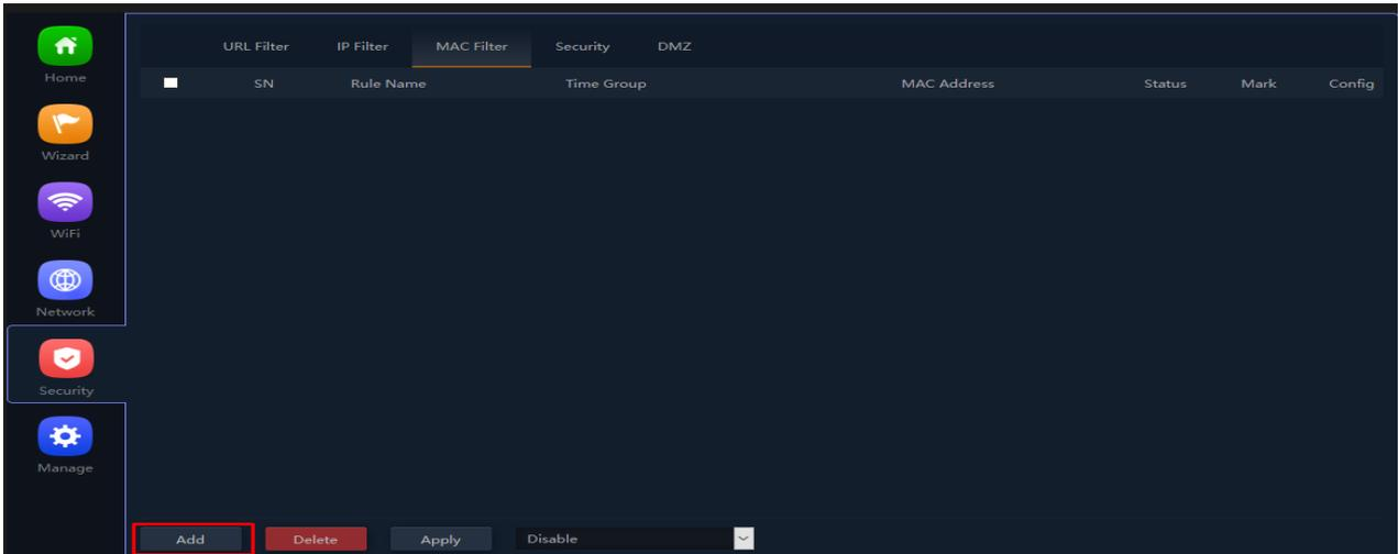
Fig 6.3.1 Default MAC filter setting for AirONE AIR-CPE1K+
