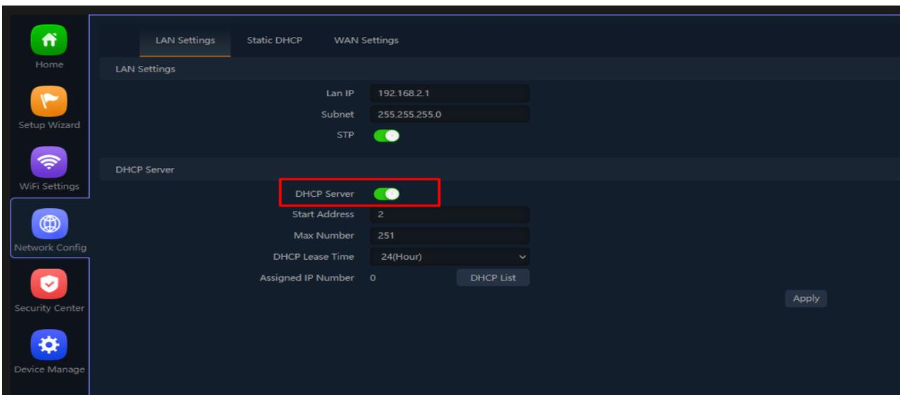
Fig 5.1.2 Setting DHCP for AirONE AIR-CPE1K+
