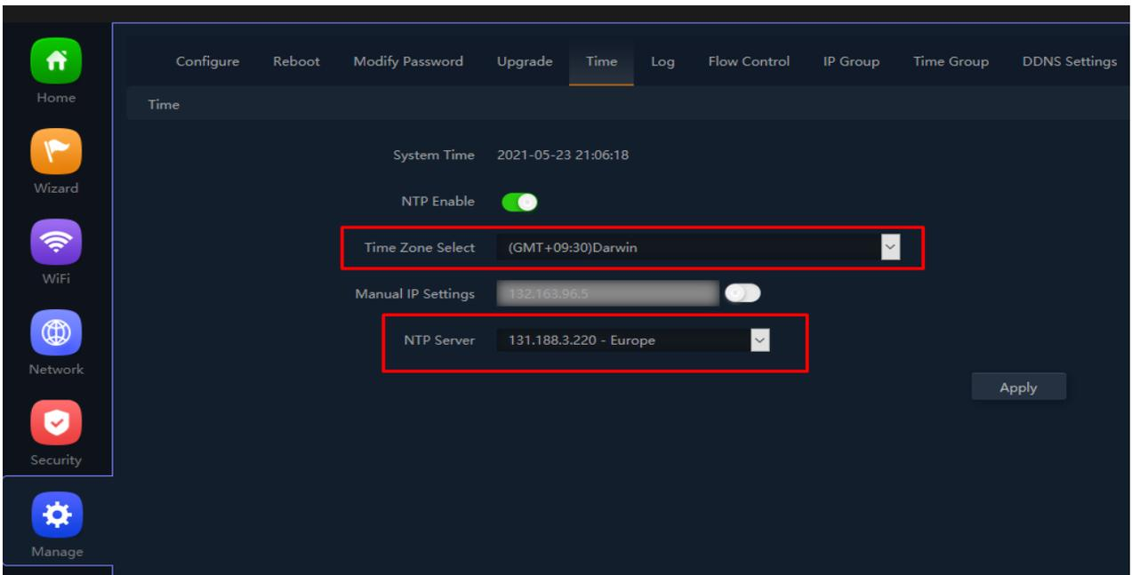
Fig 7.5.6 NTP server for AirONE AIR-CPE1K+
