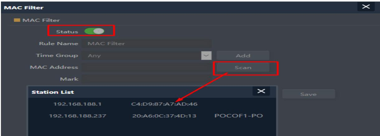
Fig 6.3.2 Setting MAC filter for AirONE AIR-CPE1K+
