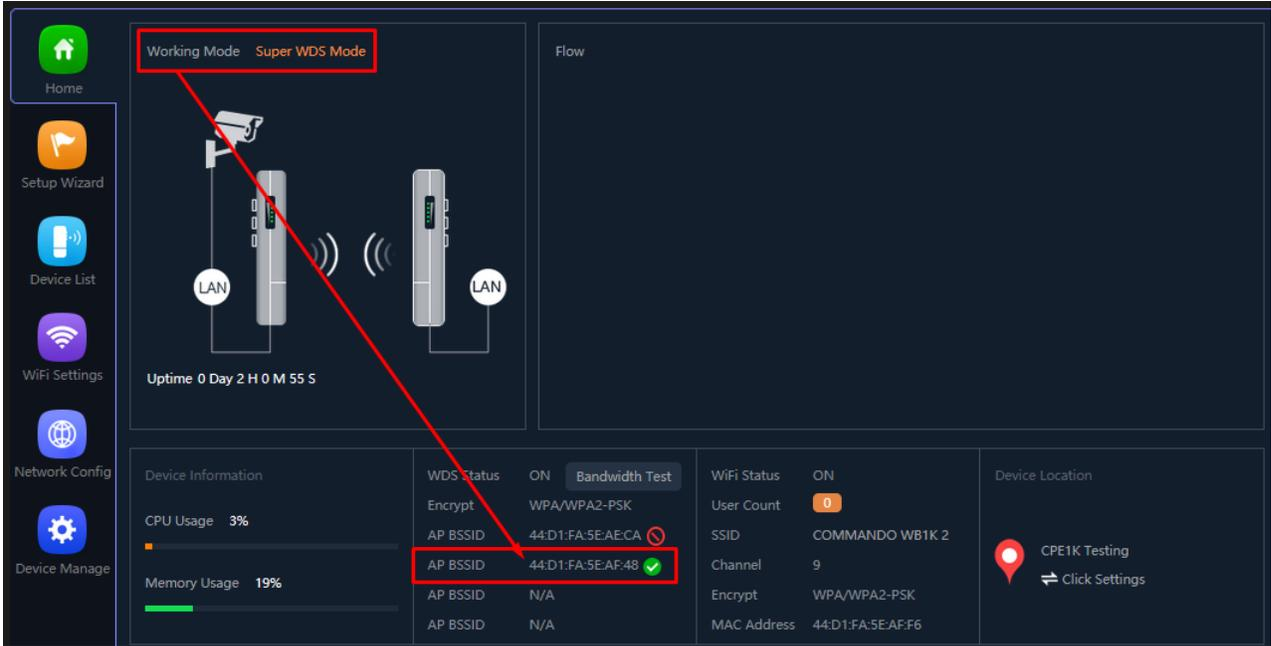
Fig 2.2.6 Active Super WDS mode of AirONE AIR-CPE1K+
