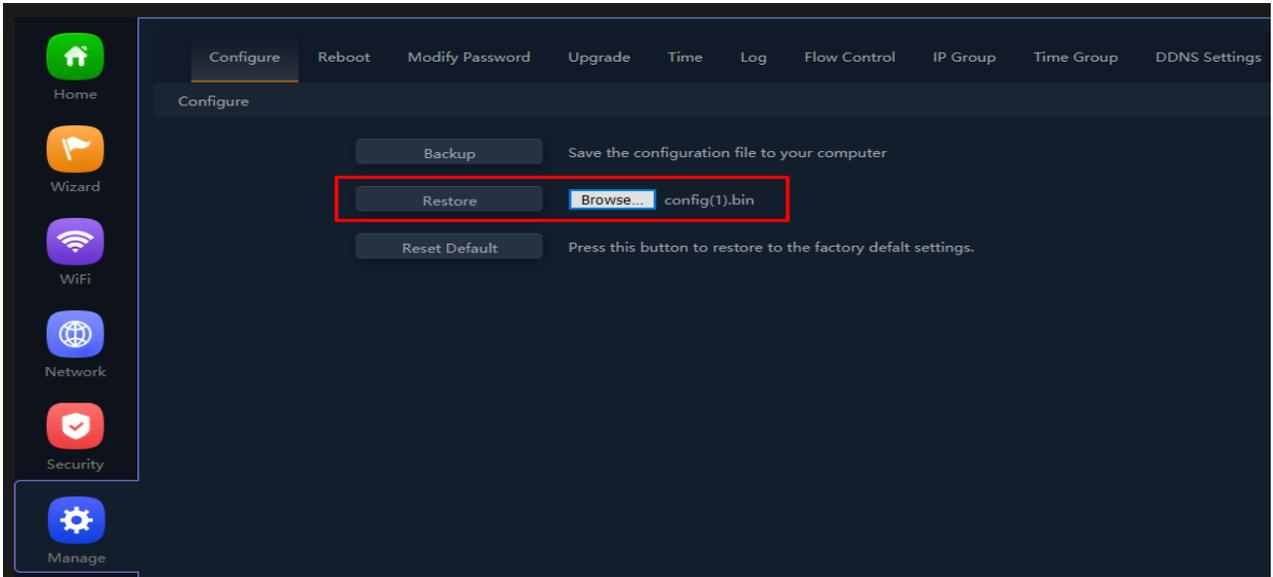
Fig 7.1.3 Restore to known Configure for AirONE AIR-CPE1K+
