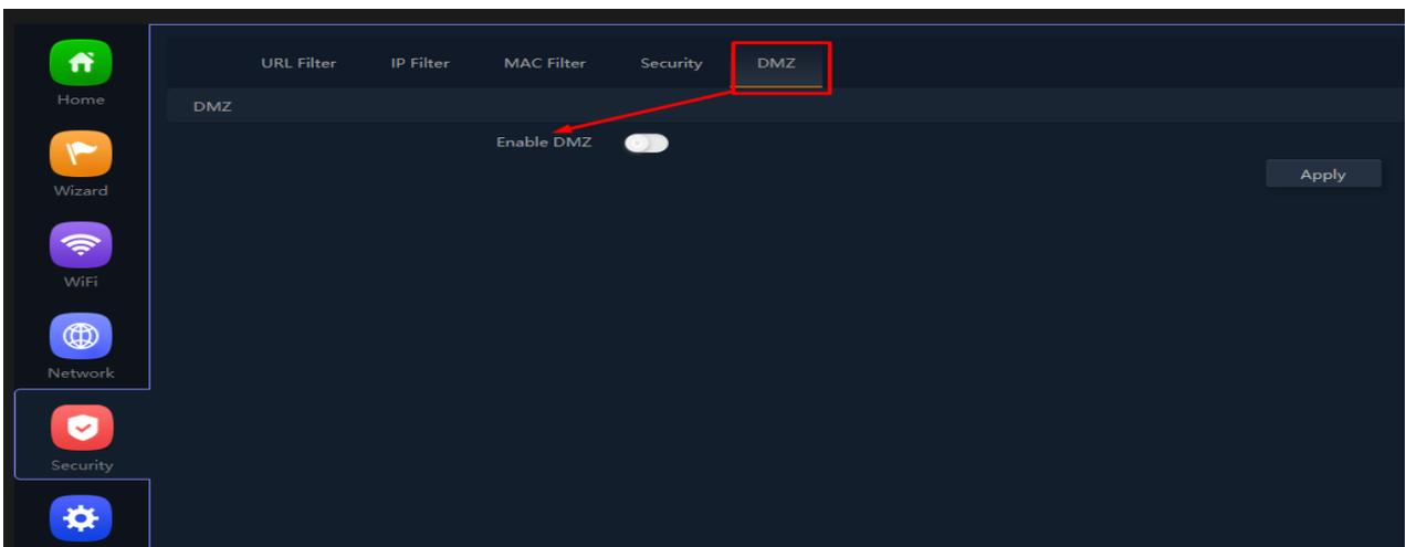
Fig 6.5.1 Default DMZ setting for AirONE WB300-1K
