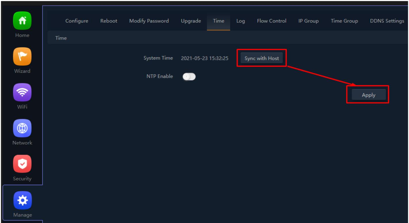
**Fig 7.5.2 Disable NTP and Sync with host for AirONE AIR-CPE5K+**
