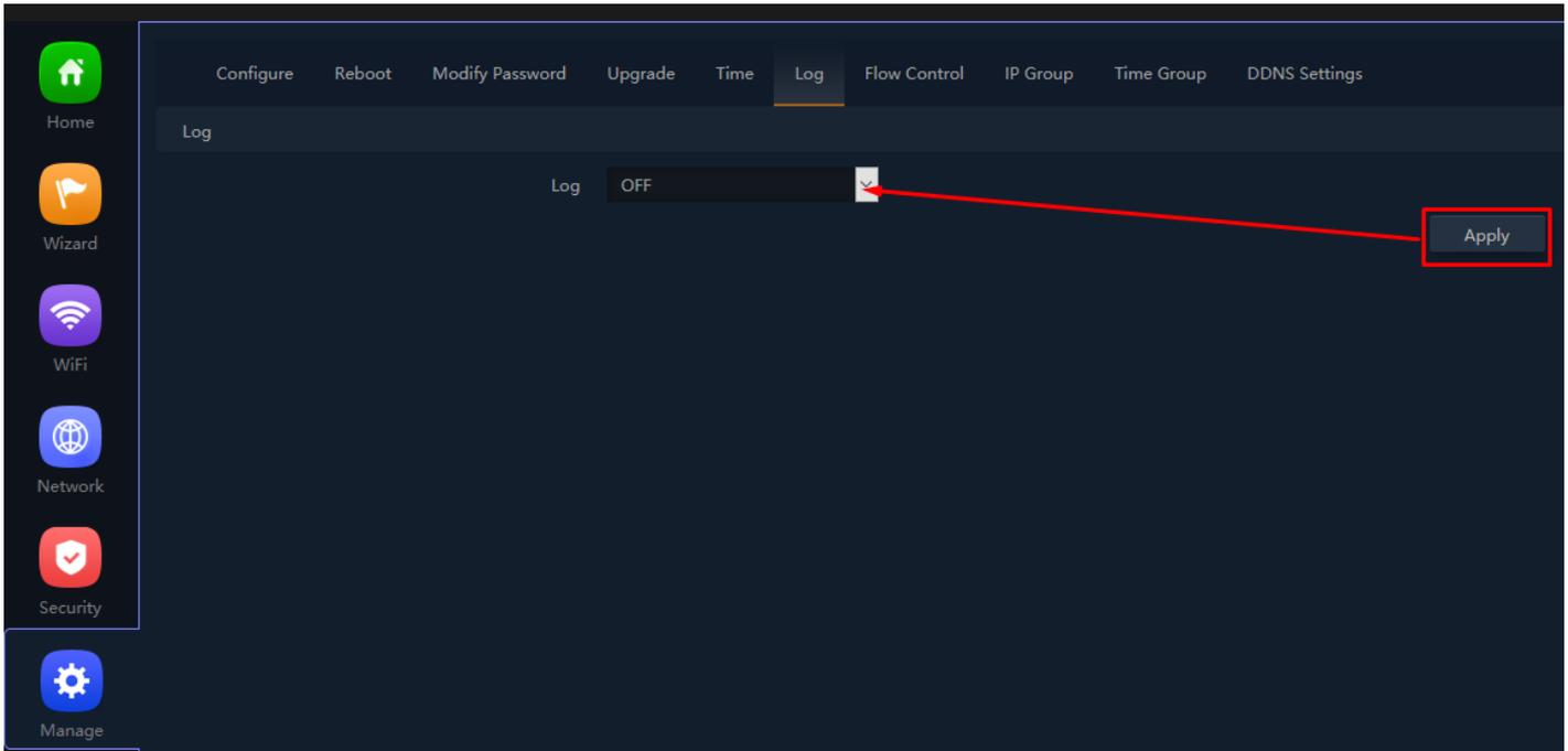
**Fig 7.6.2 Turning OFF Log setting for AirONE AIR-CPE5K+**
