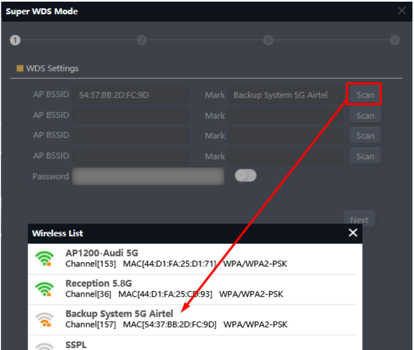
Fig 2.2.2 Scan (AP BSSID) Bridges/AP for connecting AirONE AIR-CPE5K+
