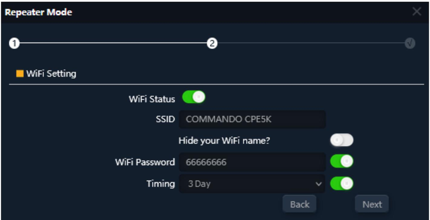
**Fig 2.3.3 Setting 5G Wi-Fi setting of AirONE AIR-CPE5K+**
