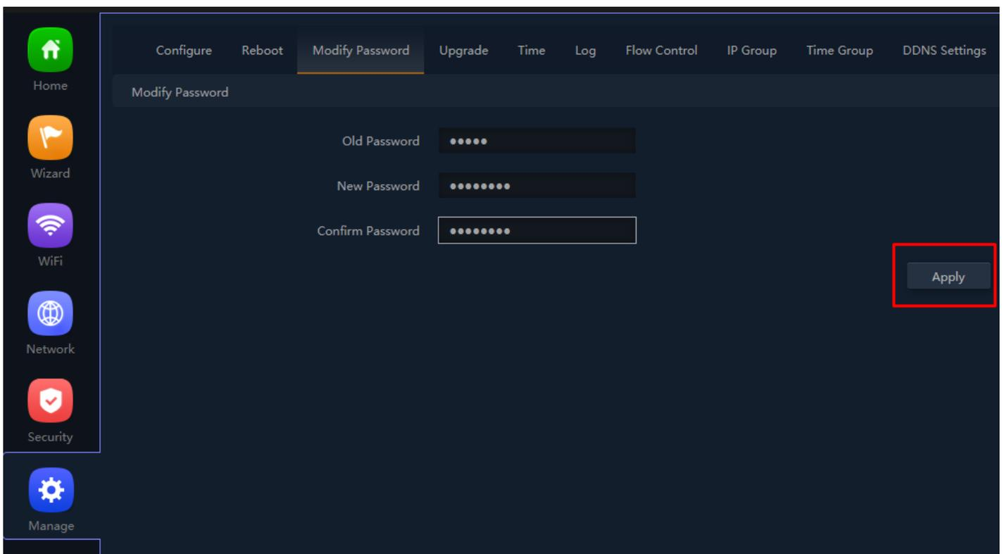
**Fig 7.3.2 Setting New password for AirONE AIR-CPE5K+**
