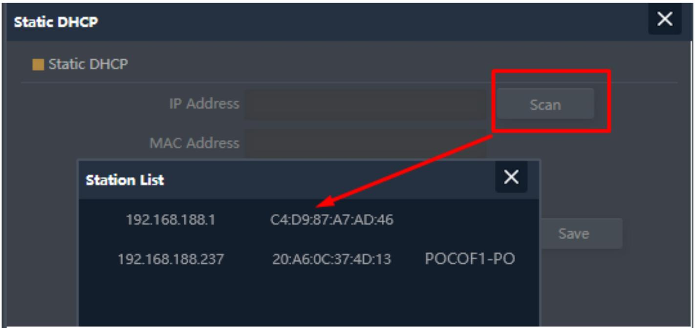
**Fig 5.3.3 Station list for AirONE AIR-CPE5K+**
