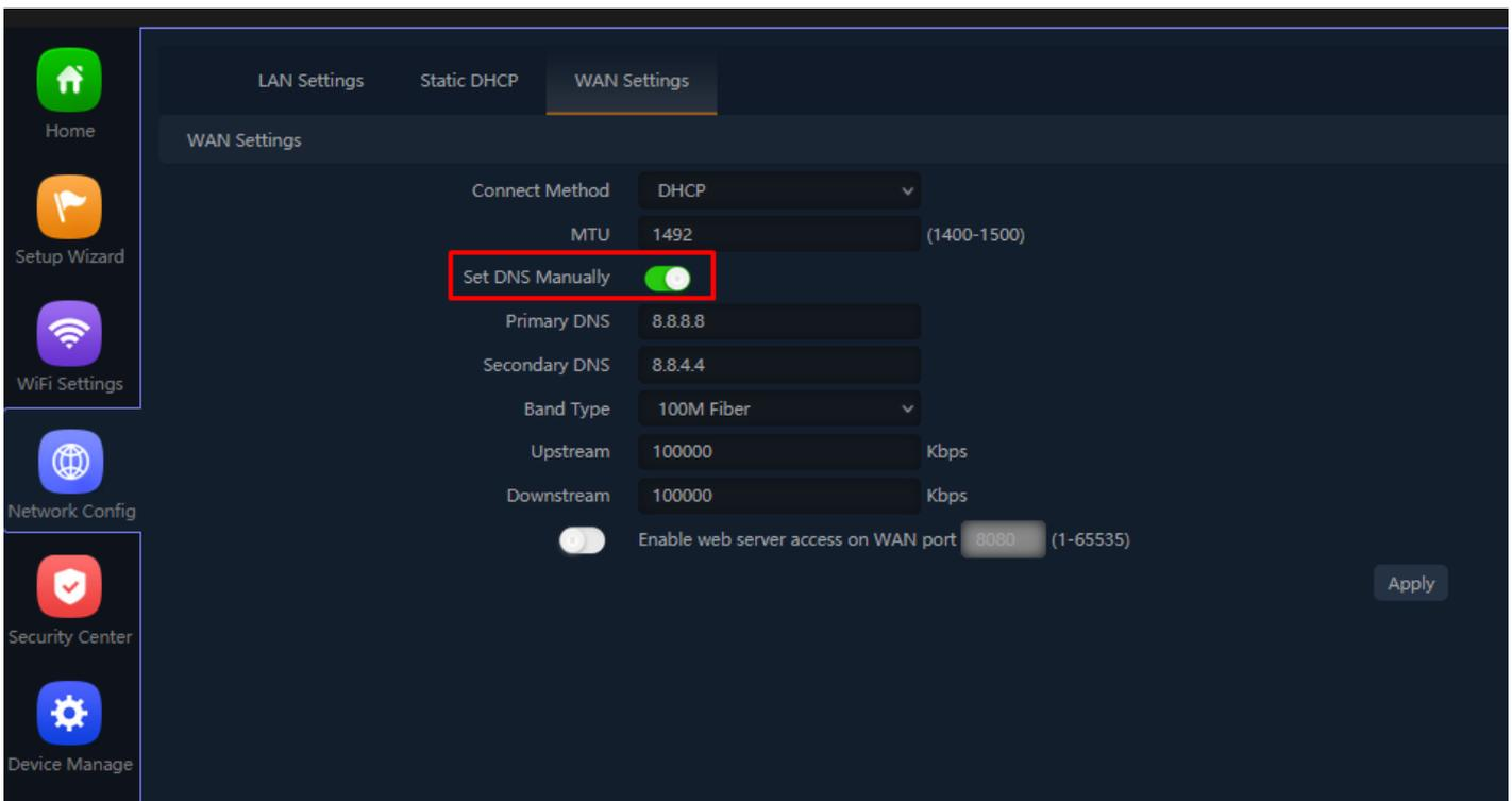
**Fig 5.4.3 Set DNS manually for AirONE AIR-CPE5K+**
