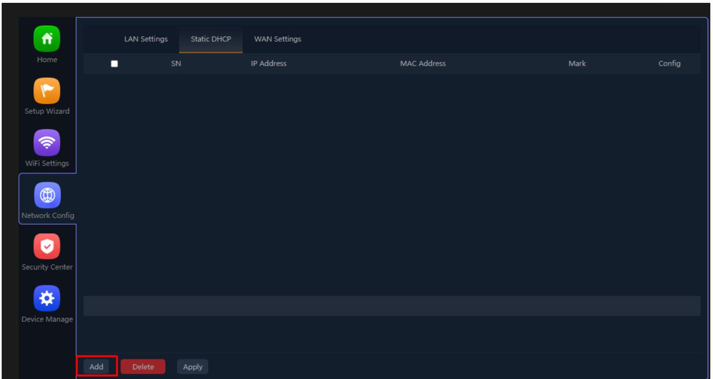
Fig 5.3.1 Default Static DHCP for AirONE AIR-CPE5K+
