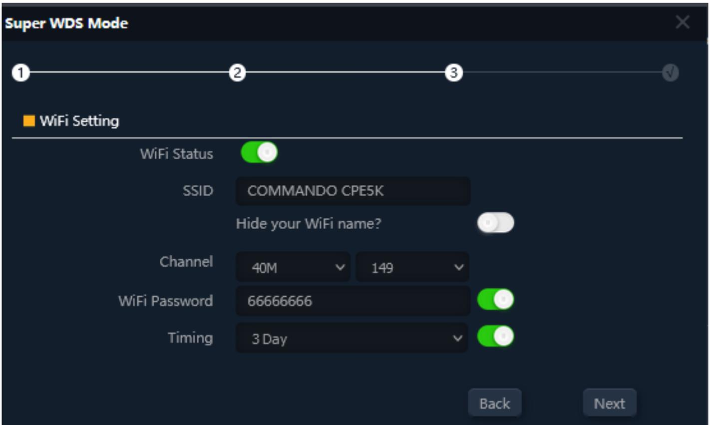
**Fig 2.2.5 Wi-Fi Setting in Super WDS mode of AirONE AIR-CPE5K+**
