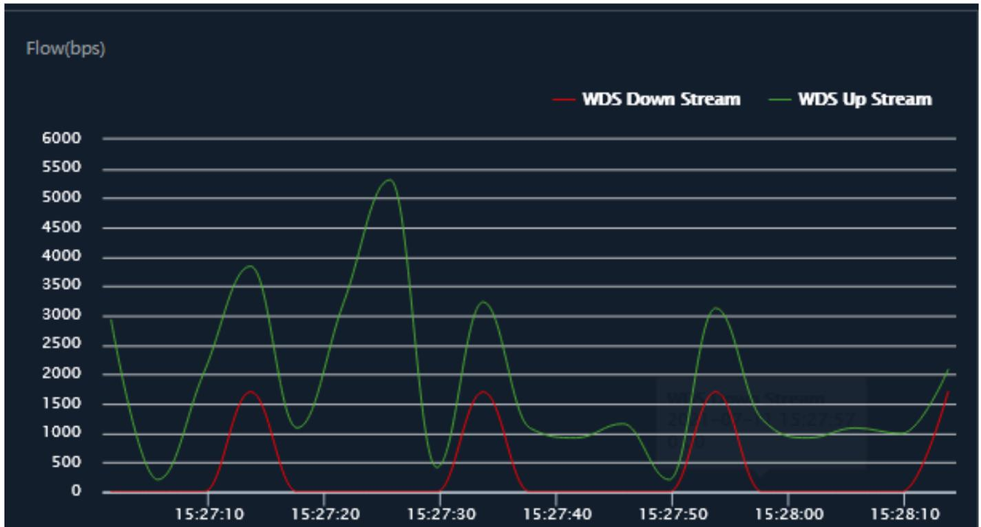
Fig 1.5.1 Flow (5G Wi-Fi) bps of AirONE AIR-CPE5K+
