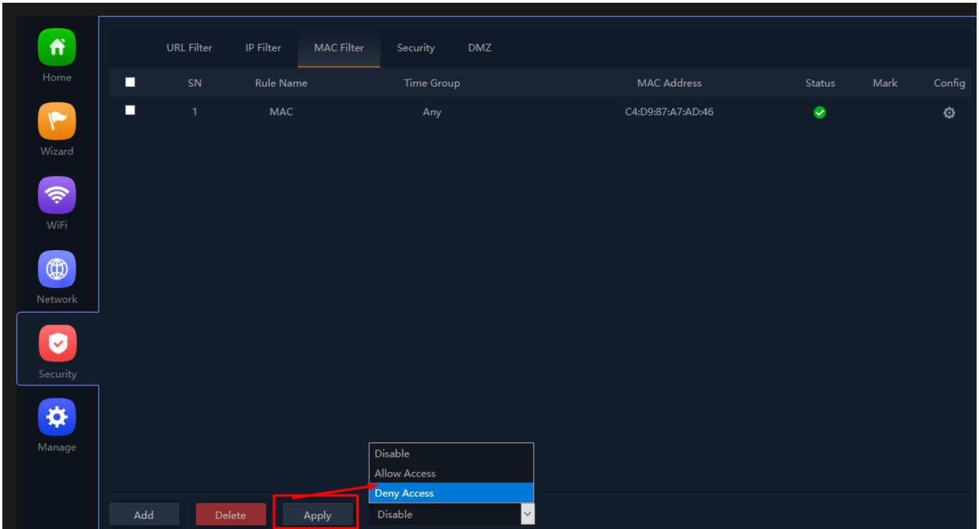
**Fig 6.3.3 MAC filter setting for AirONE AIR-CPE5K+**
