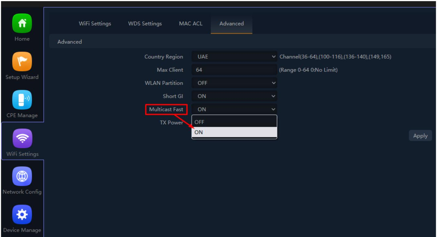
**Fig 4.4.6 Setting Multicast Fast for AirONE AIR-CPE5K+**
