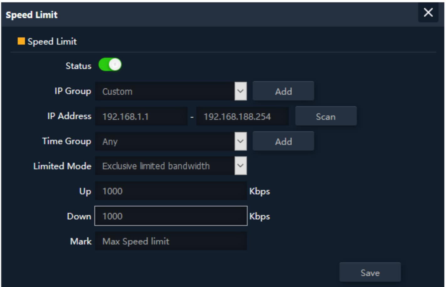
Fig 7.7.2 Enabling Speed limit for AirONE AIR-CPE5K+
