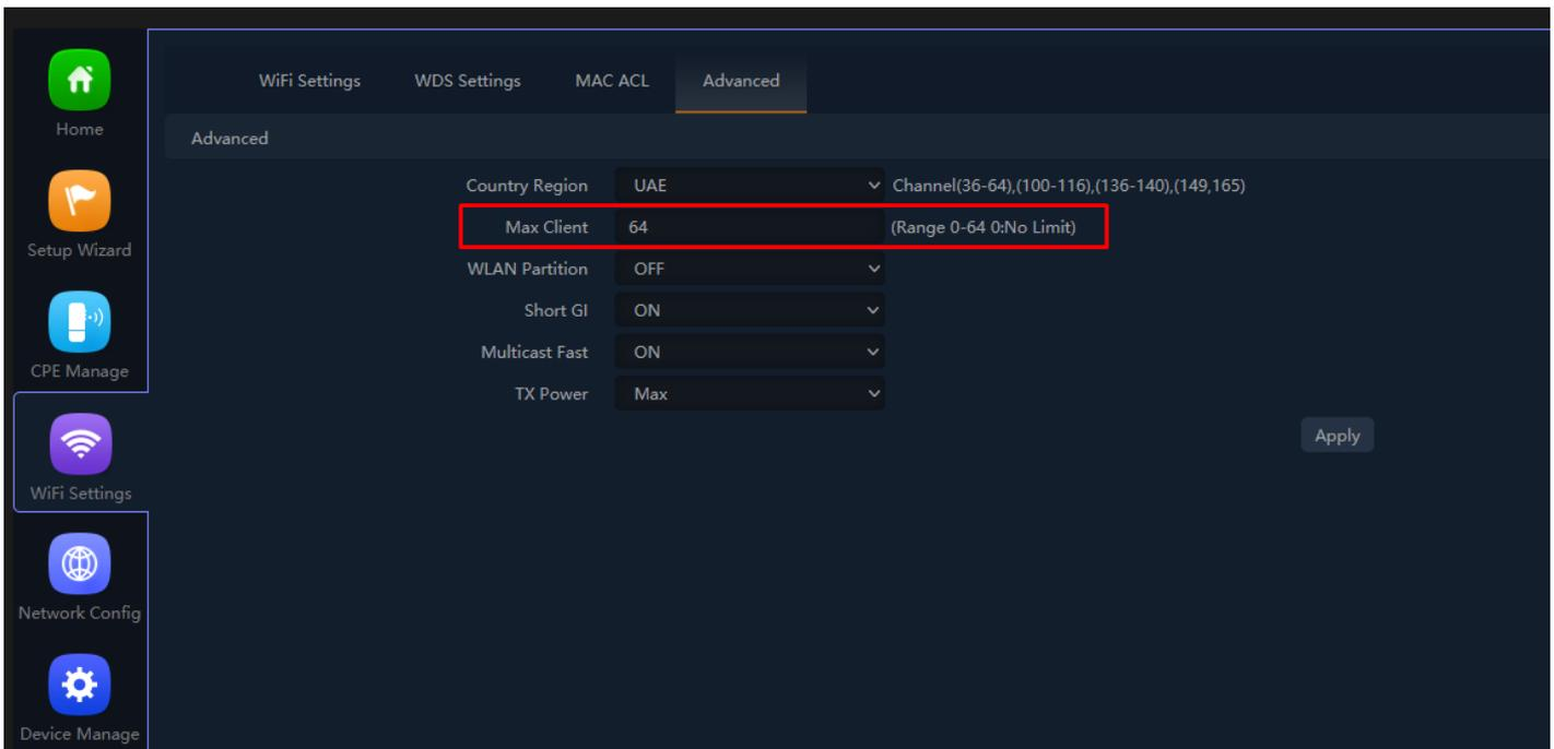
**Fig 4.4.3 Setting Maximum wireless clients in 5G for AirONE AIR-CPE5K+**
