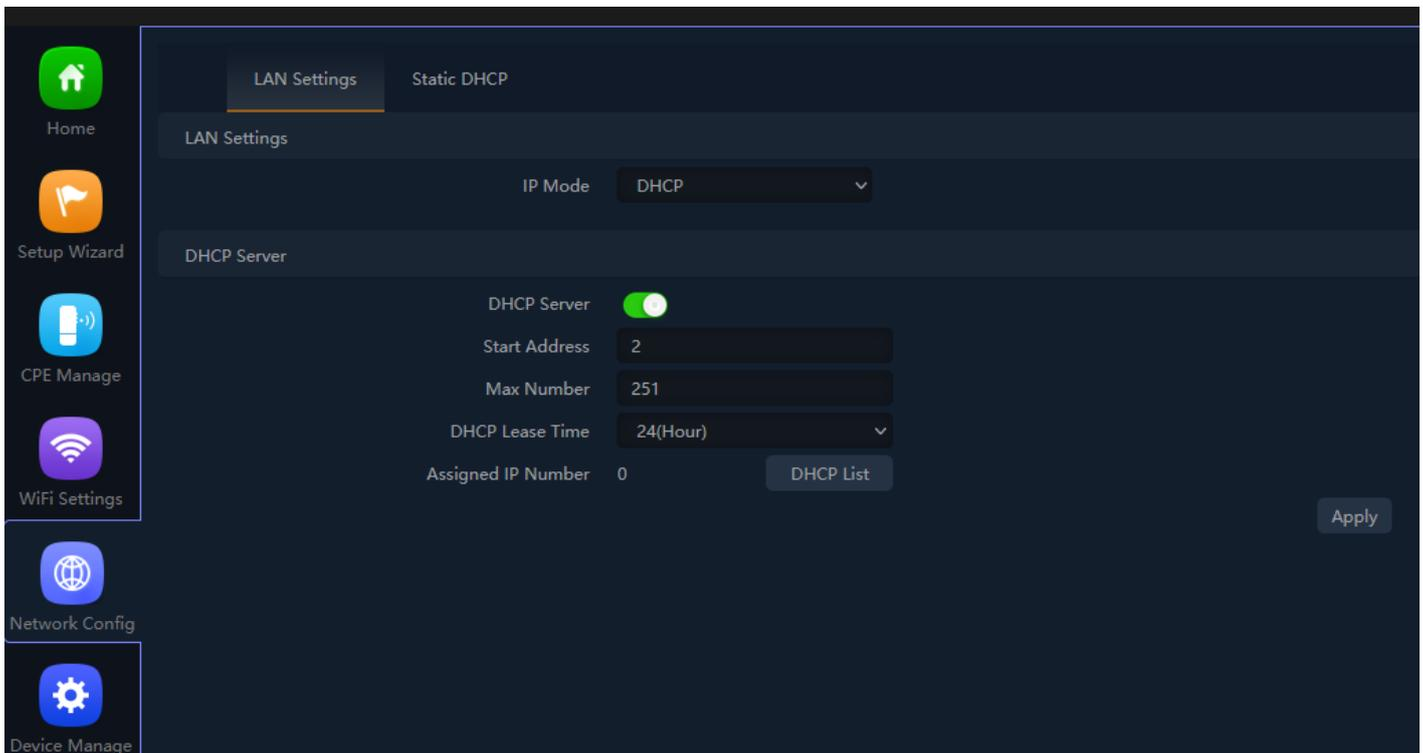
Fig 5.1.1 Setting LAN IP which used as access IP for AirONE AIR-CPE5K+
