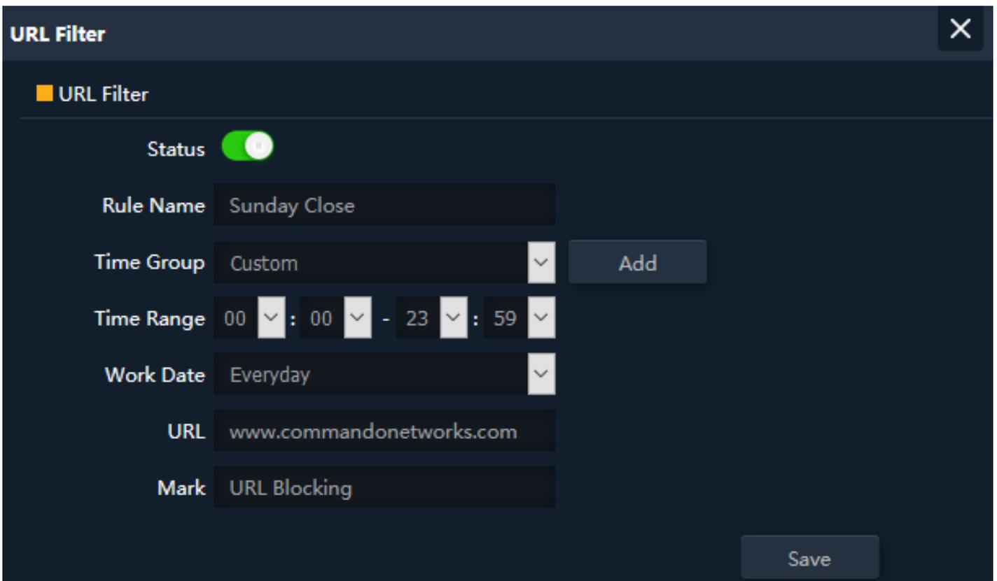
Fig 6.1.2 Setting URL filter for AirONE AIR-CPE5K+
