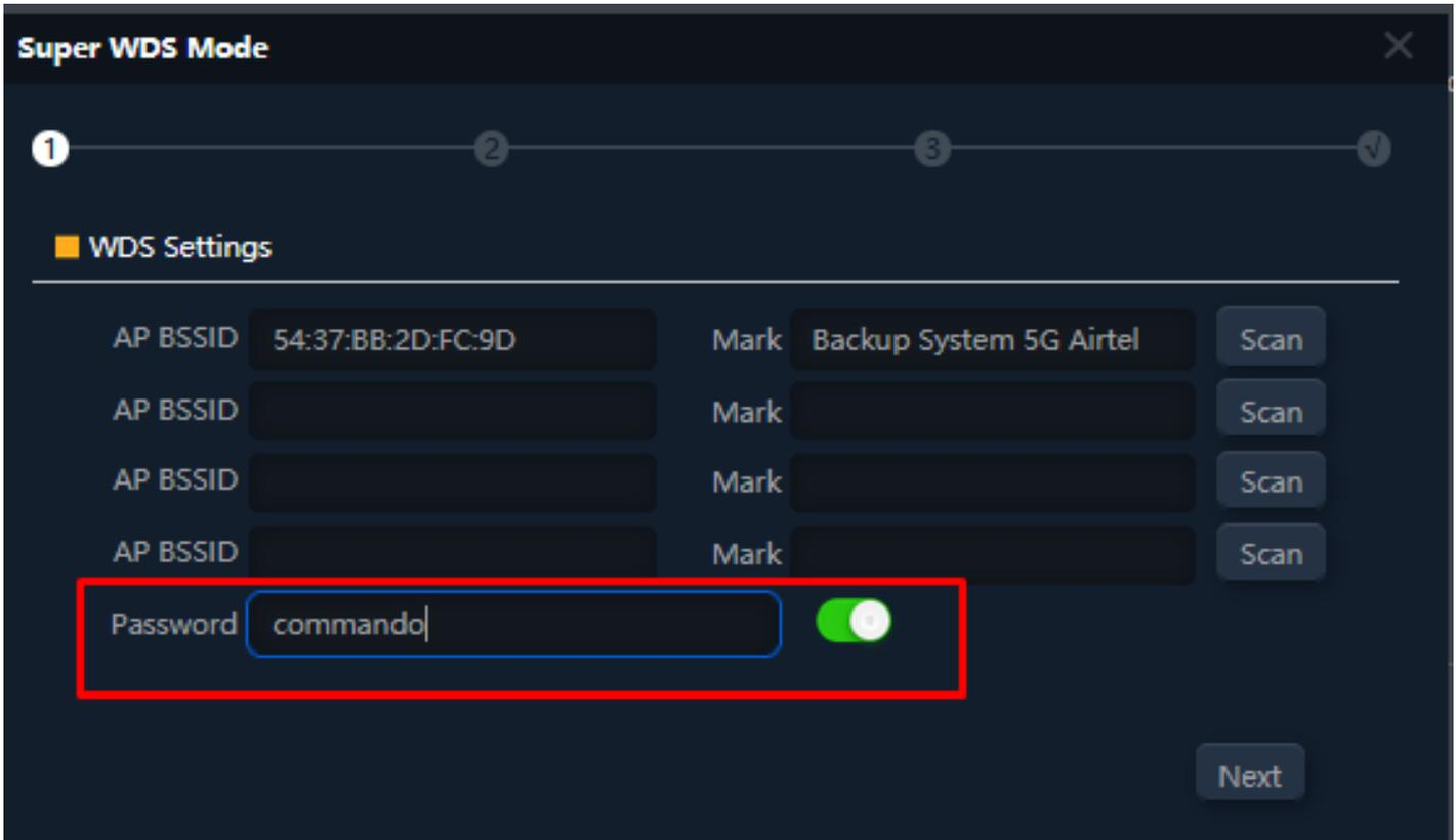
Fig 2.2.3 Super WDS mode scan Bridges/ SSID for AirONE AIR-CPE5K+
