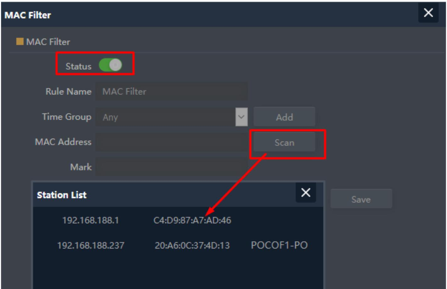
**Fig 6.3.2 Setting MAC filter for AirONE AIR-CPE5K+**
