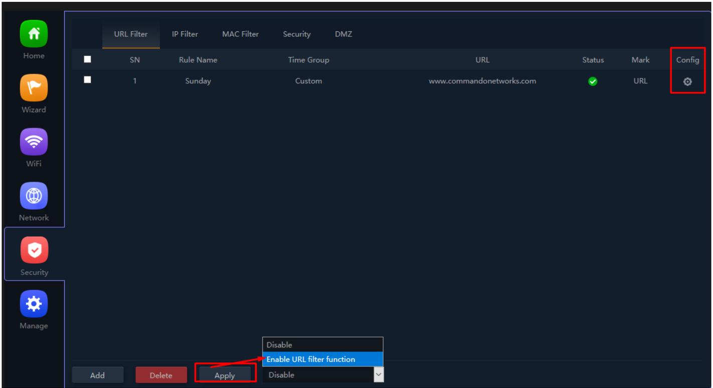
**Fig 6.1.3 URL filter setting for AirONE AIR-CPE5K+**
