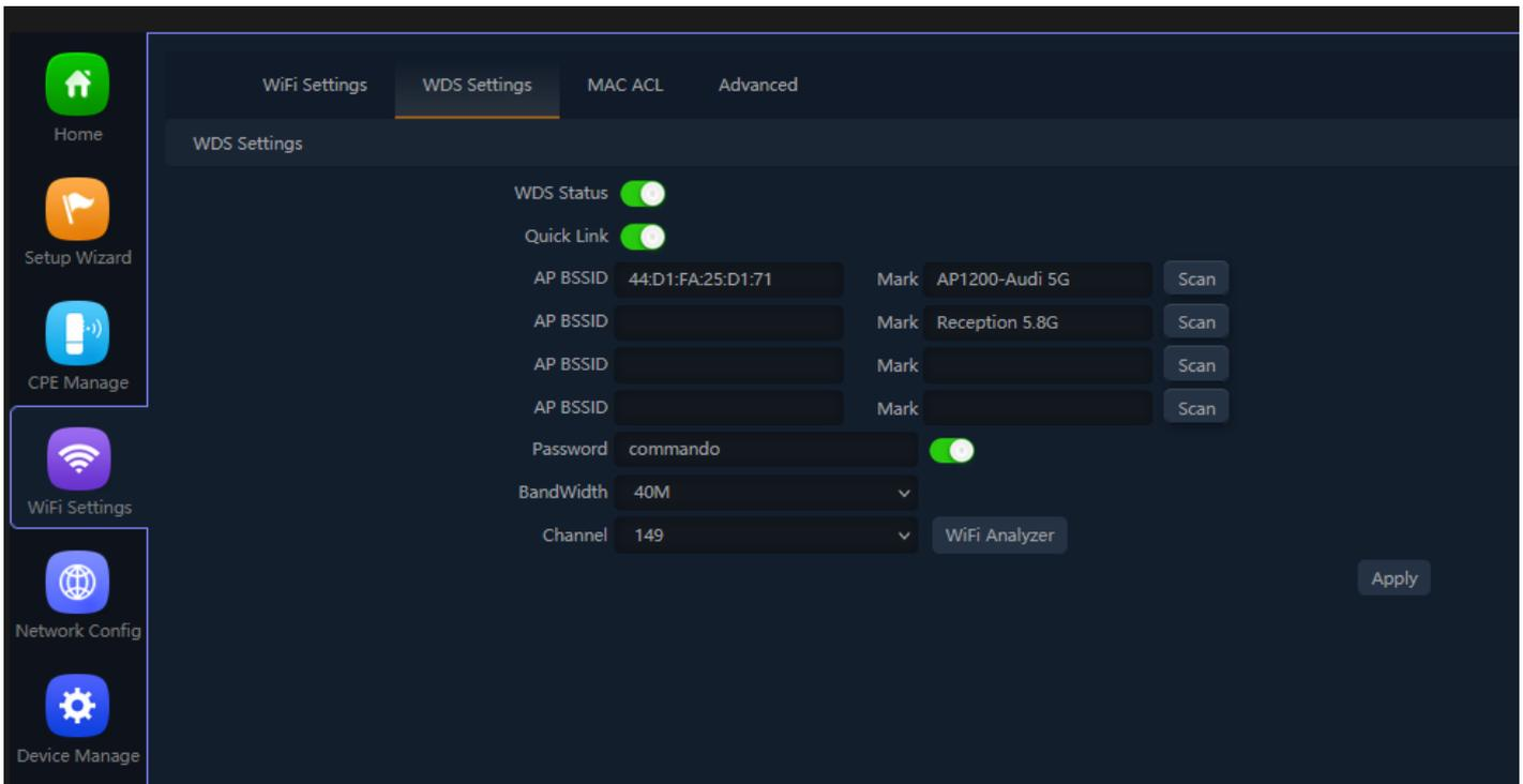
**Fig 4.2.1 WDS Setting for AirONE AIR-CPE5K**
