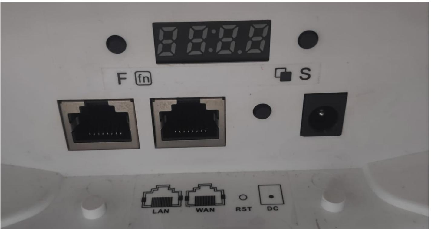
**Fig 1. Physical port on AirONE AIR-CPE5K+**
