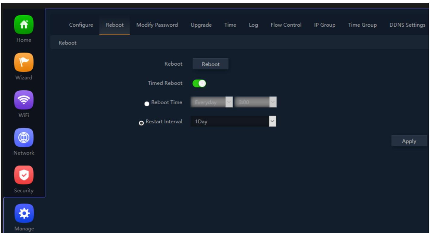
**Fig 7.2.5 Enable Restart interval for AirONE AIR-CPE5K+**
