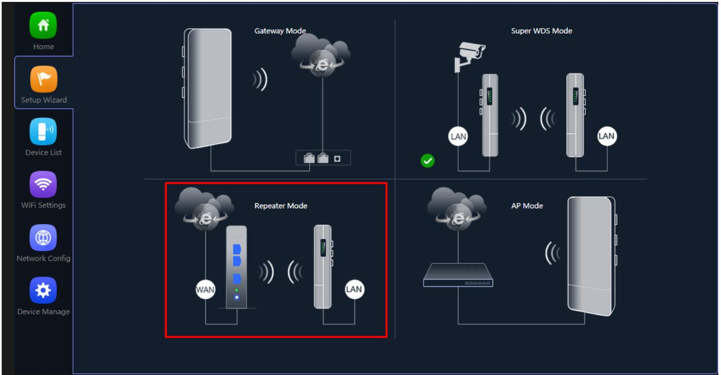
**Fig 2.3.1 Repeater mode of AirONE AIR-CPE5K+**
