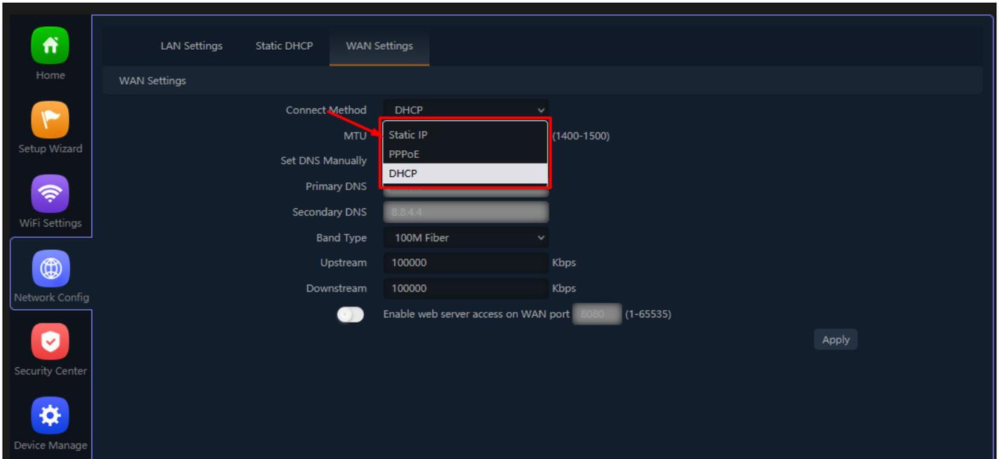
**Fig 5.4.2 Changing Connect type manually for AirONE AIR-CPE5K+**
