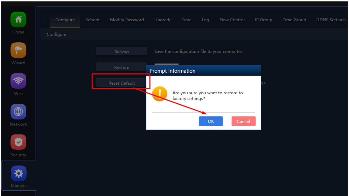
**Fig 7.1.4 Reset to factory default for AirONE AIR-CPE5K**
