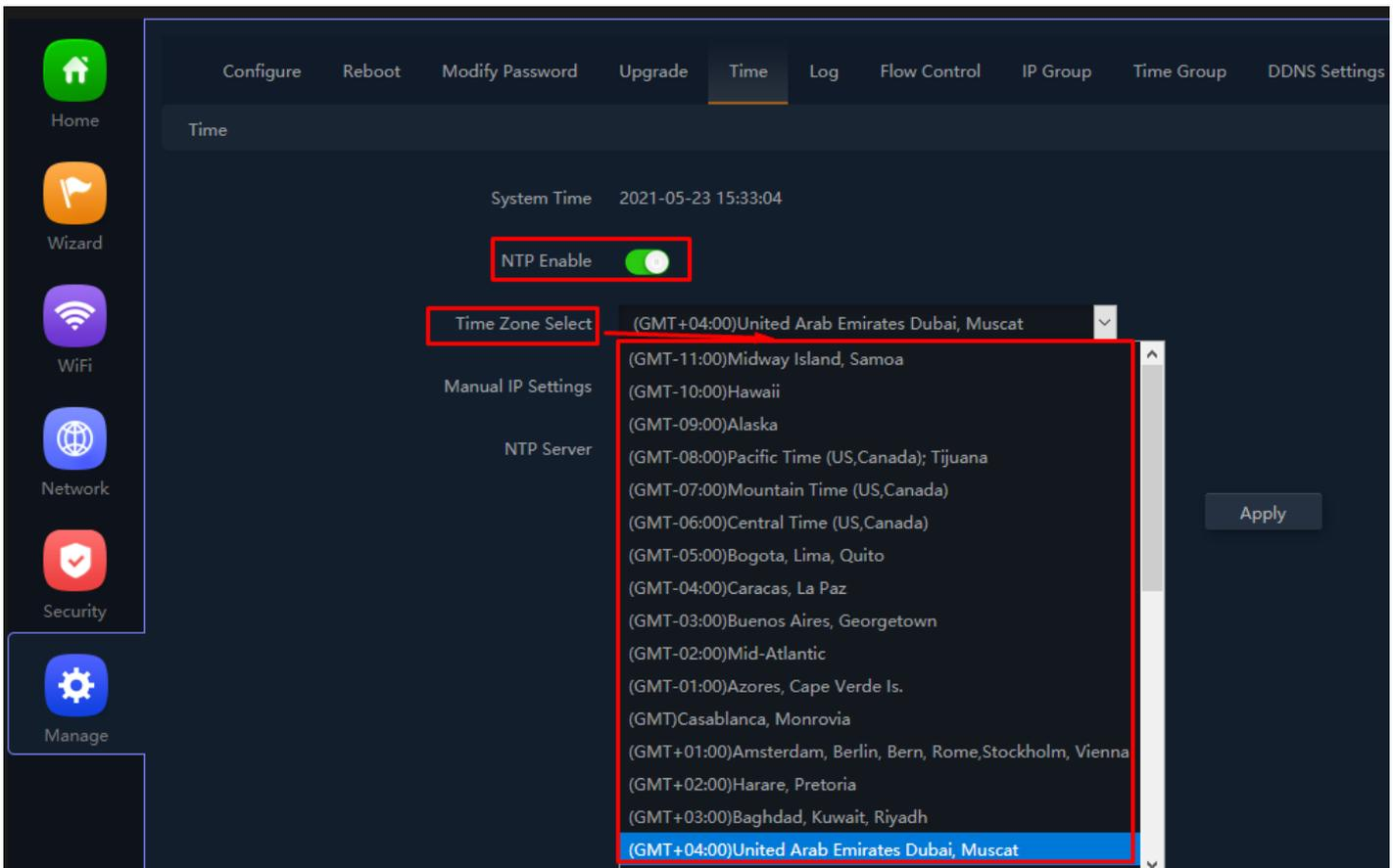
**Fig 7.5.3 Enable NTP and select time zone for AirONE AIR-CPE5K+**
