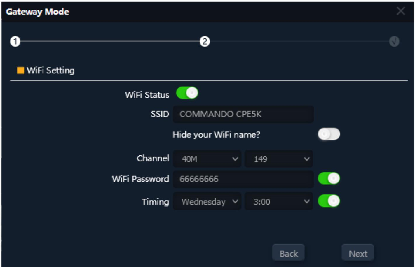
**Fig 2.1.3 Gateway mode Wi-Fi Setting of AirONE AIR-CPE5K+**
