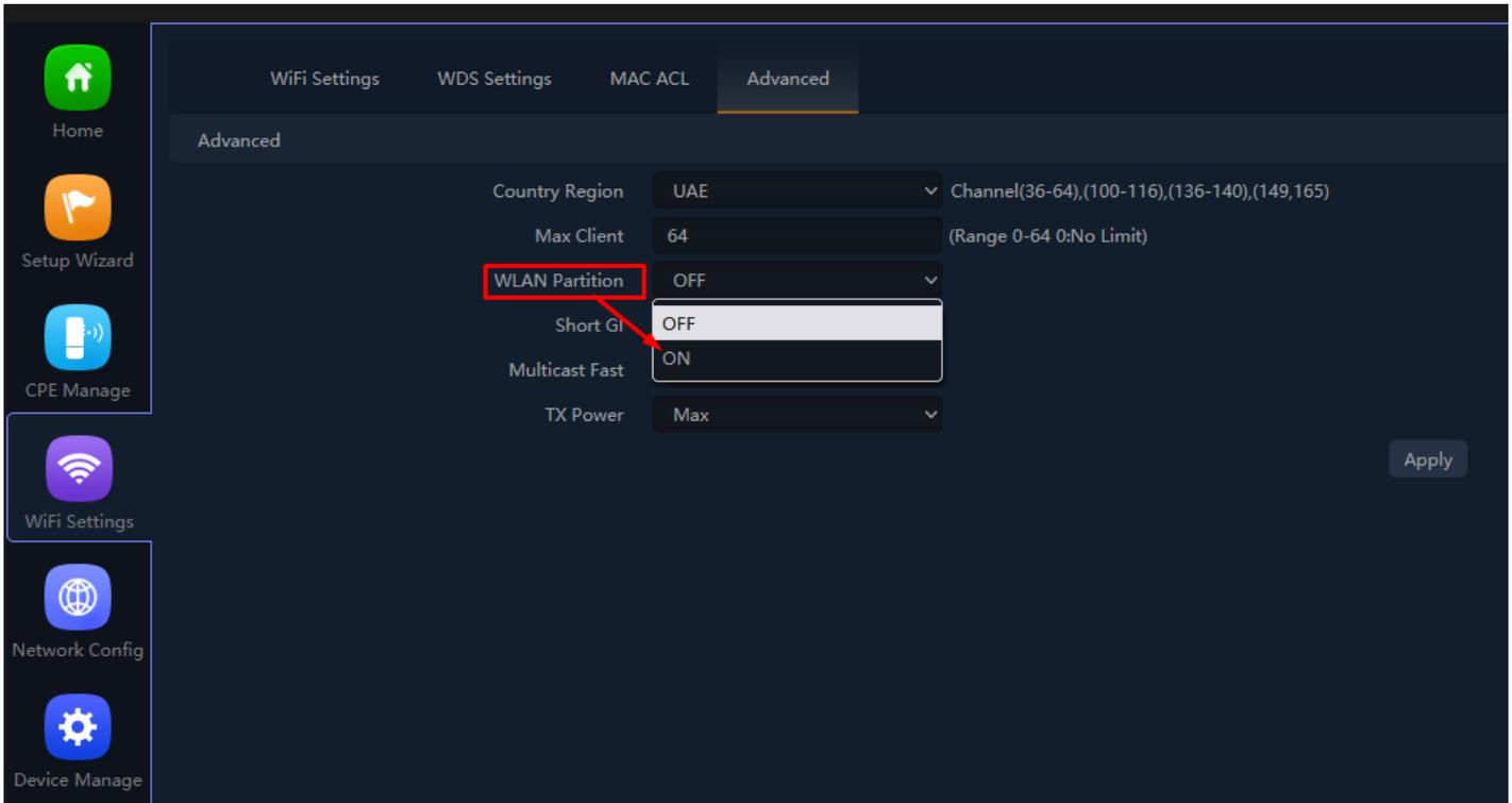
**Fig 4.4.4 Selecting WLAN Partition for AirONE AIR-CPE5K+**
