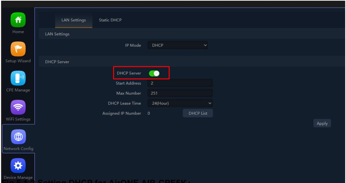
Fig 5.1.2 Setting DHCP for AirONE AIR-CPE5K+
