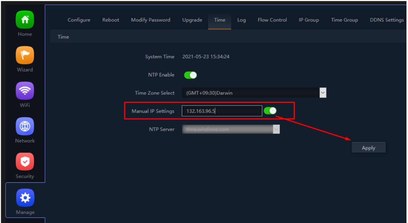
Fig 7.5.4 Enable NTP with Manual IP setting for AirONE AIR-CPE5K+
