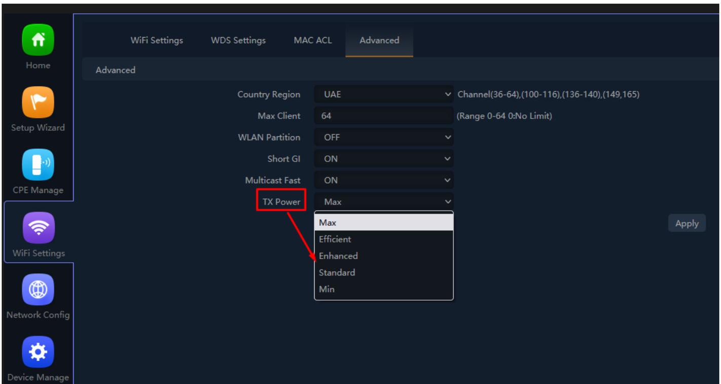
**Fig 4.4.7 Setting Tx Power for AirONE AIR-CPE5K+**
