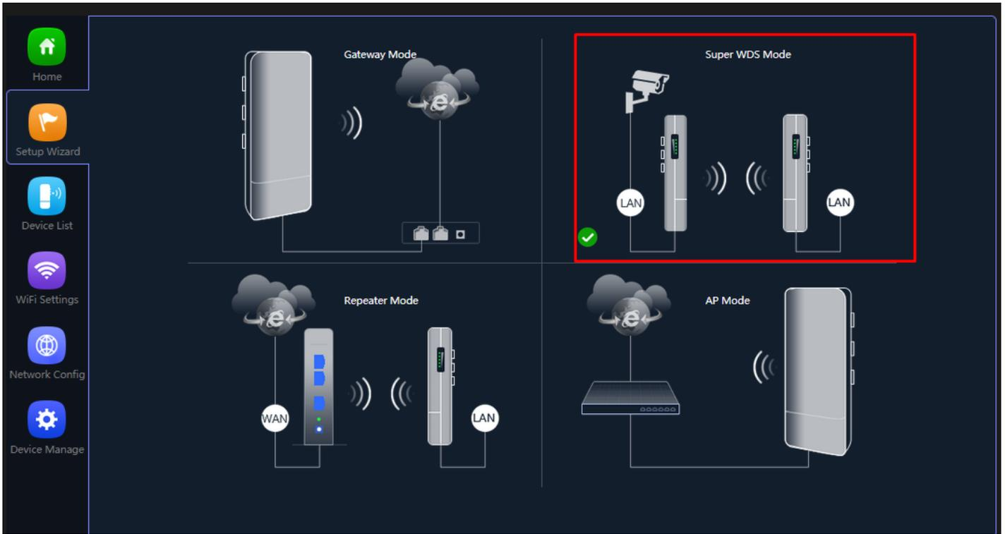
**Fig 2.2.1 Super WDS mode of AirONE AIR-CPE5K+**
