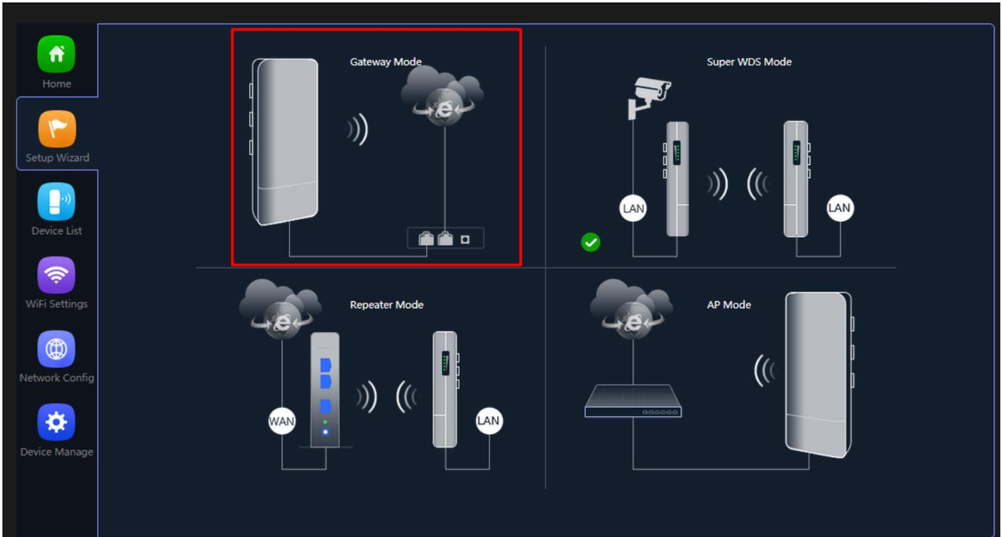
Fig 2.1.1 Gateway mode of AirONE AIR-CPE5K+
