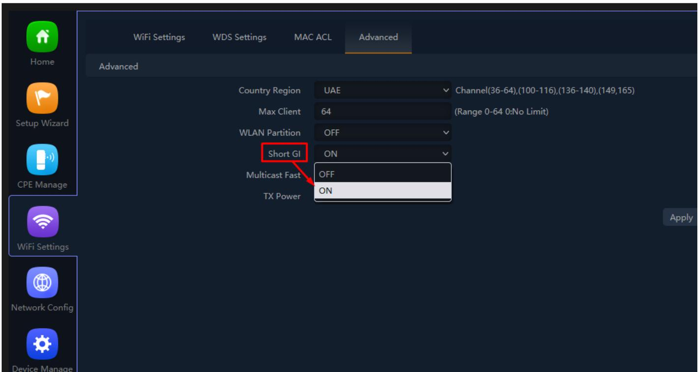
**Fig 4.4.5 Selecting Short GI for AirONE AIR-CPE5K+**
