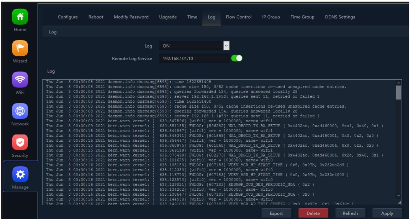
**Fig 7.6.4 Enabling Remote Log server setting IP for AirONE AIR-CPE5K+**
