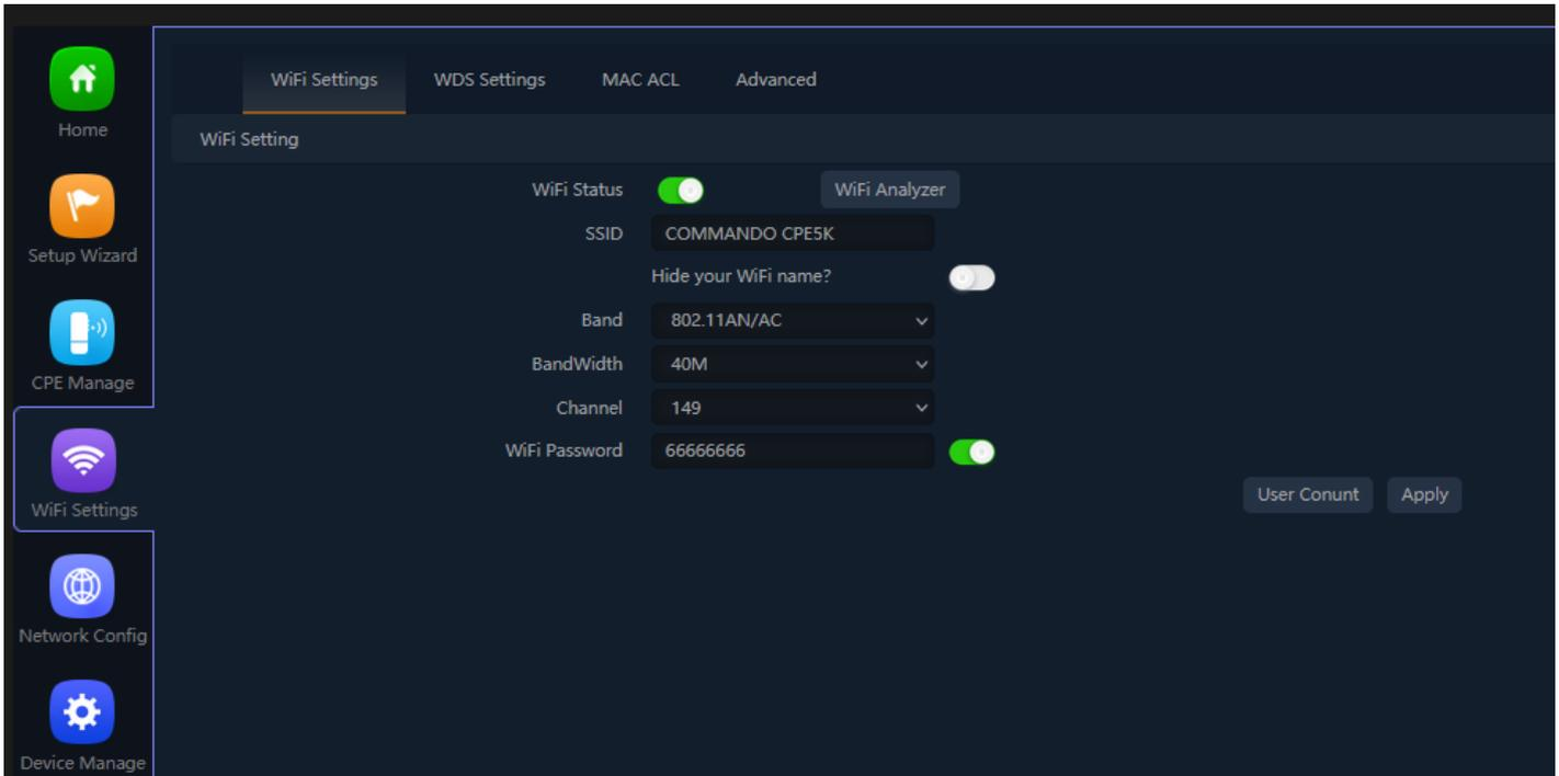
**Fig 4.1.1 Wi-Fi setting of AirONE AIR-CPE5K+**
