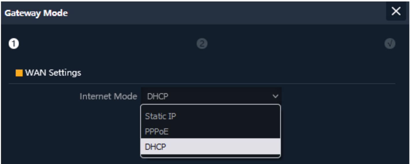
Fig 2.1.2 Gateway mode WAN Setting of AirONE AIR-CPE5K+
