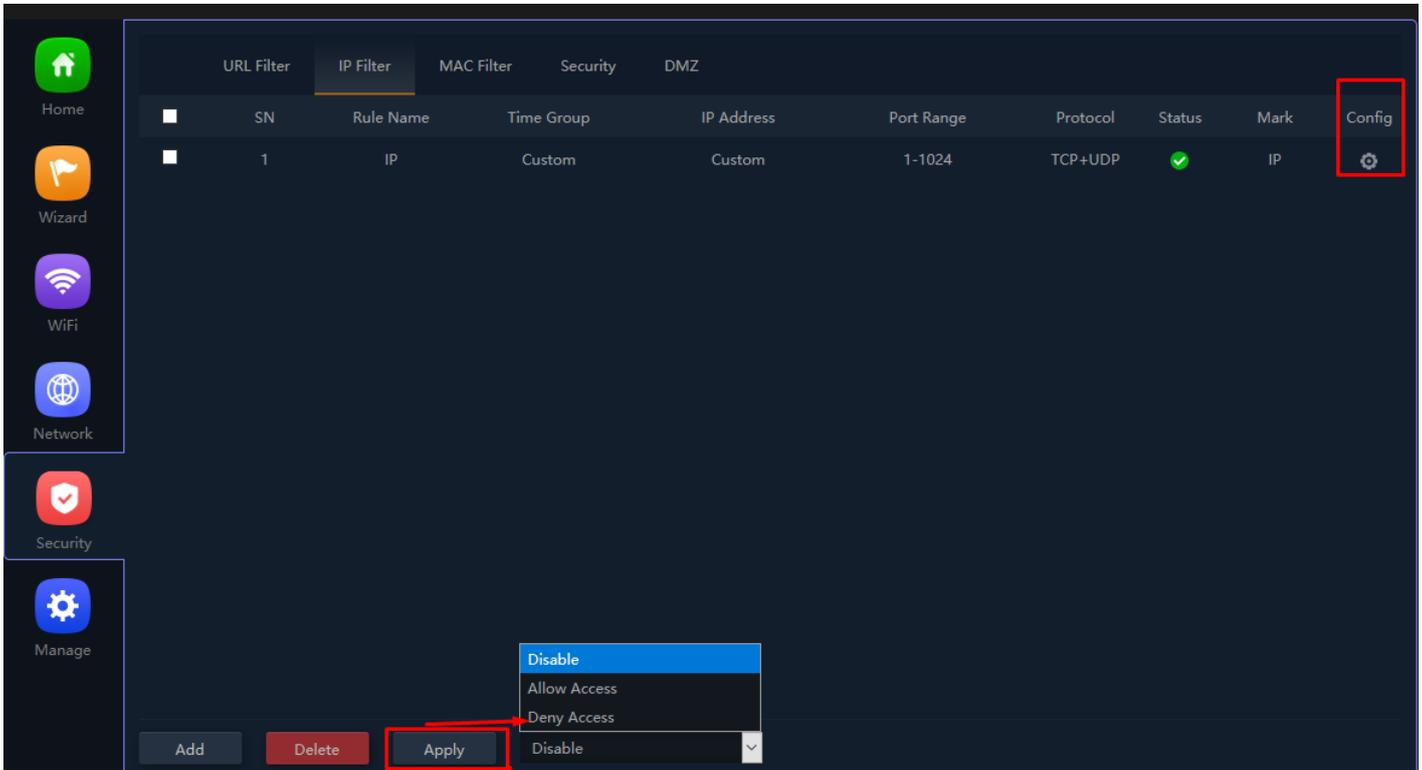
**Fig 6.2.3 IP filter setting for AirONE AIR-CPE5K+**
