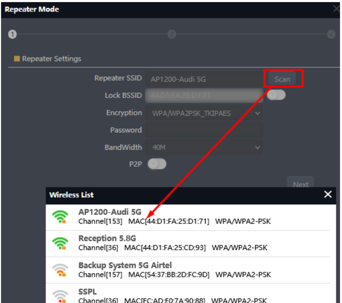
Fig 2.3.2 Selecting Repeater SSID of AirONE AIR-CPE5K+
