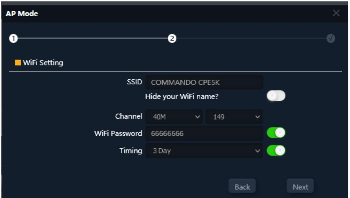
**Fig 2.4.3 Setting 5G Wi-Fi for AP mode of AirONE AIR-CPE5K+**
