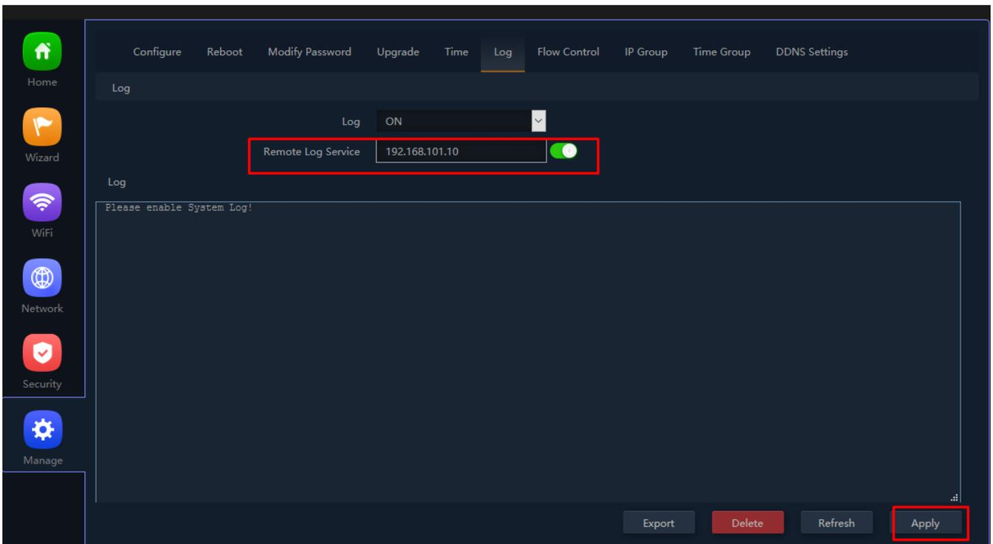
**Fig 7.6.3 Remote Log service setting IP for AirONE AIR-CPE5K+**
